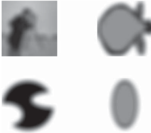
Figure 3.3: Smoothed images from Figure 3.2 using a 15 \times 15 Gaussian filter with standard deviation of 5 pixels.
