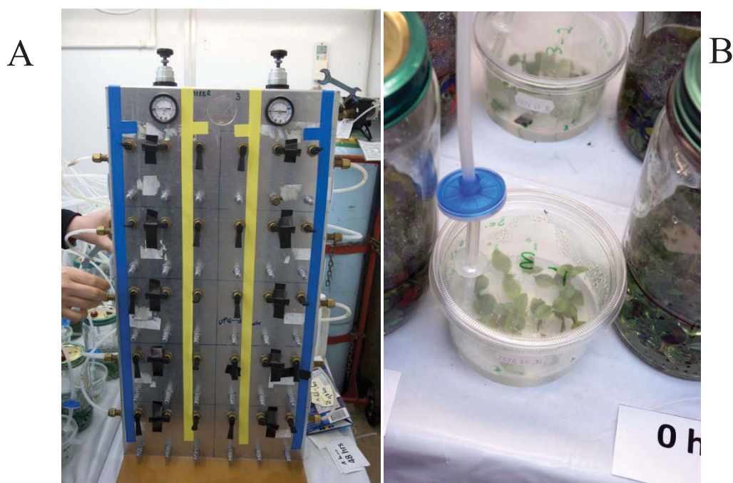
Figure 5-3: (A) Manifold for distributing the gas to vessels; (B) External gas was filtered to remove microorganisms before getting into the culture vessels.
