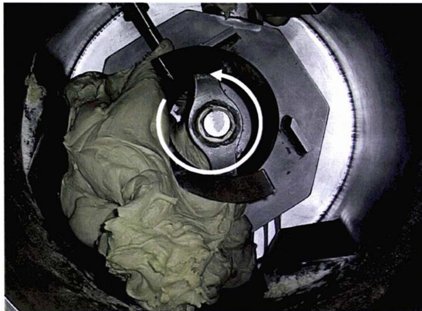
Figure 2.5 Picture of ECS 35 mixer. Arrow indicates direction of blade motion.
