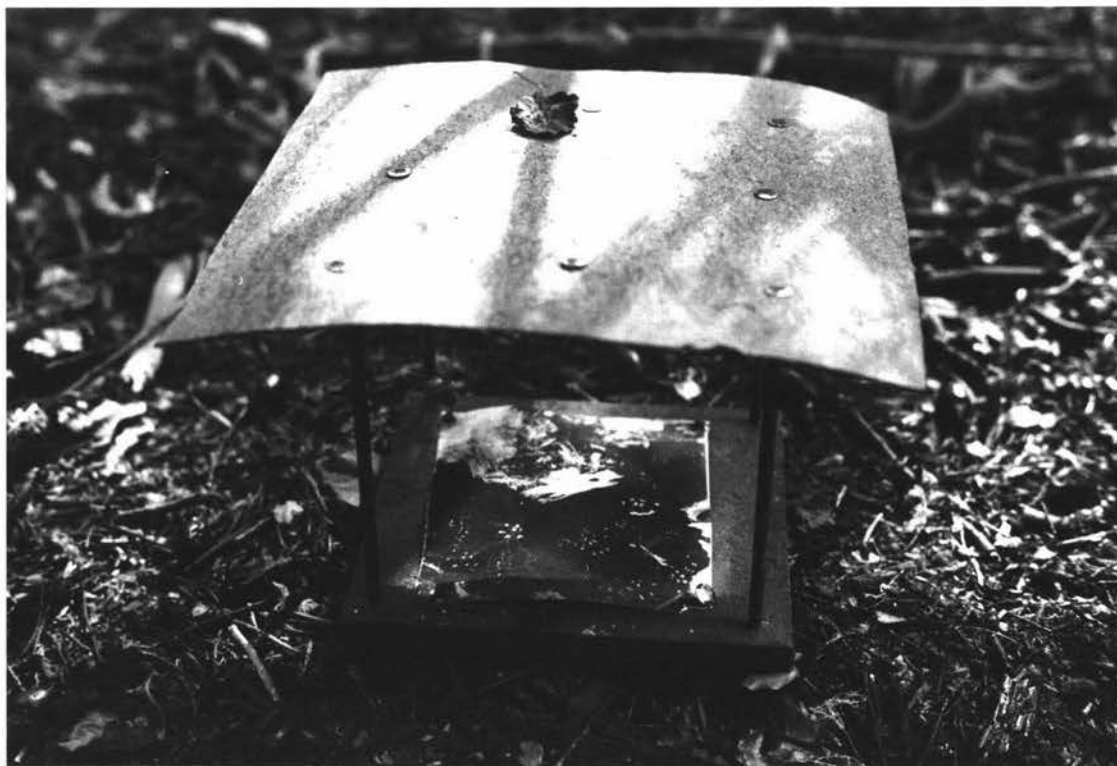
Plate 17: Device to record prints of mammals visiting an exclosure
