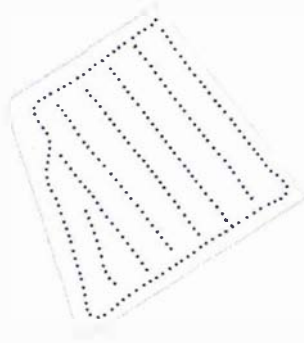
Figure 7.1. Collected GPS track log from a Bredal K65-1134 dual spinning disc fertiliser spreader using RINEX GuideTrax software on a 3.48 ha paddock.
