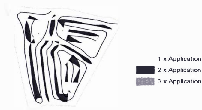
Figure 5.2. Output from Basic spreader interpolation data showing areas receiving single and double application rates using a Bredal spreader with a 26 m bout width.
