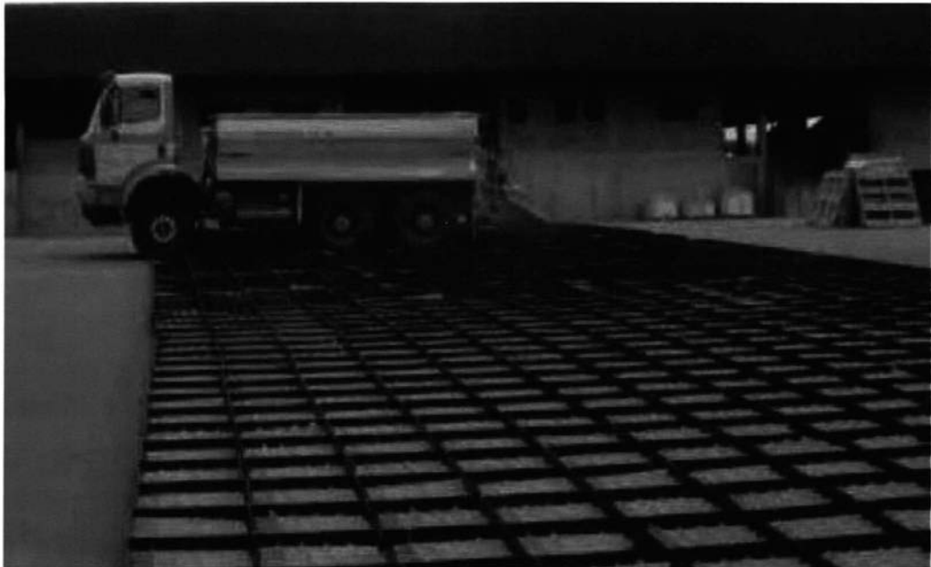
Figure 2.1. 1400 Tray matrix used to collect 18 simultaneous transverse tests on a Transpread W twin chain spreader.
