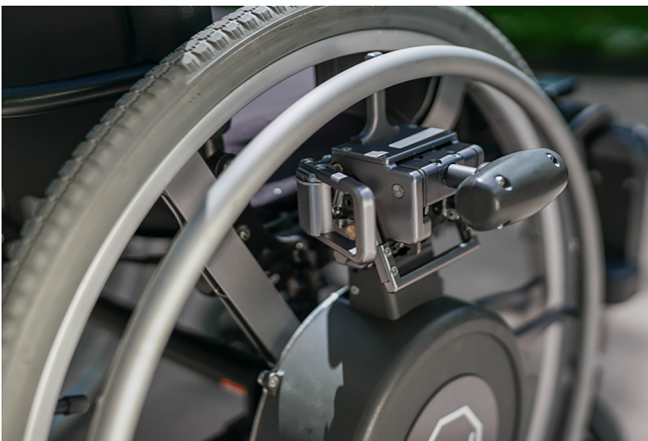
Figure 3. Bi-modal wheel in Run mode with the handle unfurled.
