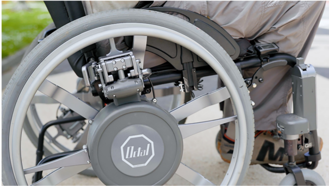
Figure 2. Bi-modal wheel in Standard mode with the handle furled.
