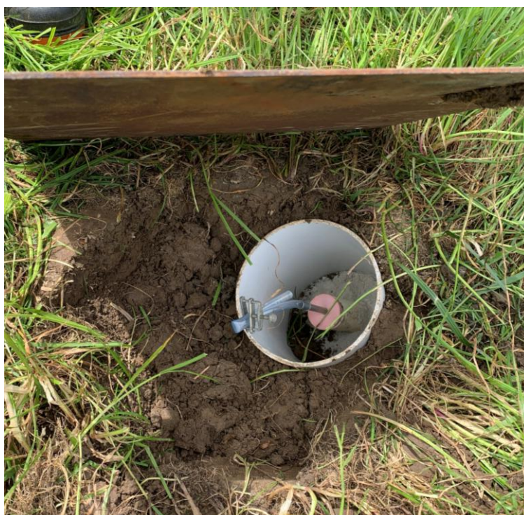
Figure 13: An example of the suction cup set-up prior to installation (left) and post-installation in the field at Moutoa (right).
