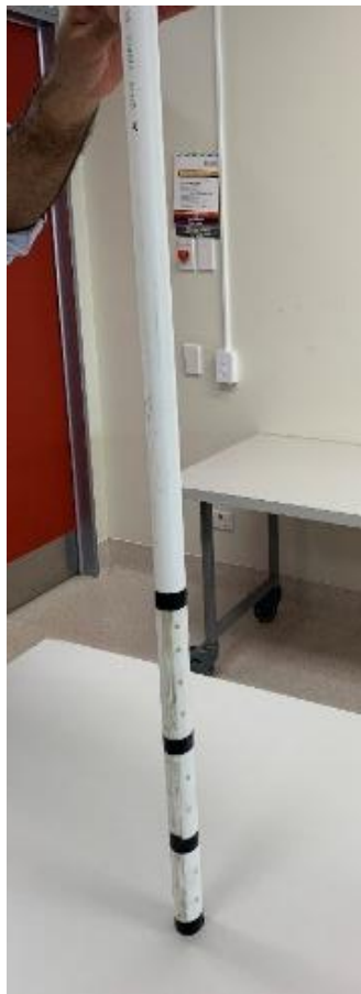
Figure 11: A sample section of piezometer pipe, showing the screen at the bottom, consisting of drilled holes and mesh.
