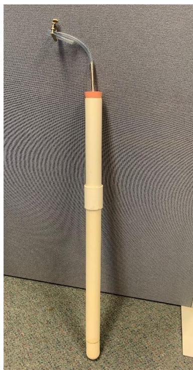
Figure 13: An example of the suction cup set-up prior to installation (left) and post-installation in the field at Moutoa (right).
