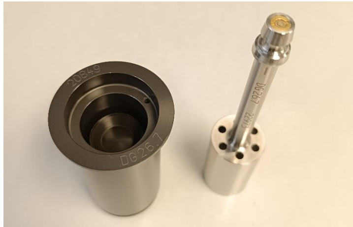
The double gap geometry used for viscosity measurements
