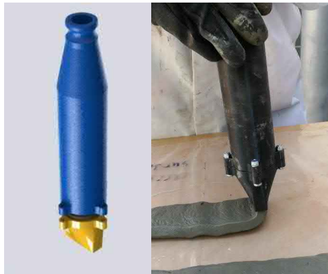
Figure 1 - (Left) Expanded view of the modular extruder assembly, (Right) Hand printing concrete using 3D printed extruder assembly with the nuzzle of 40 x 10 mm.
