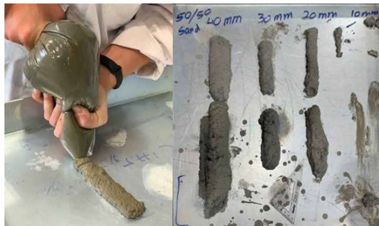
Figure 4 – (Right) Manually extrusion of a concrete mixture using a plastic bag for concrete workability test, (Left) Sample result for a mixture using different nuzzle sizes.
