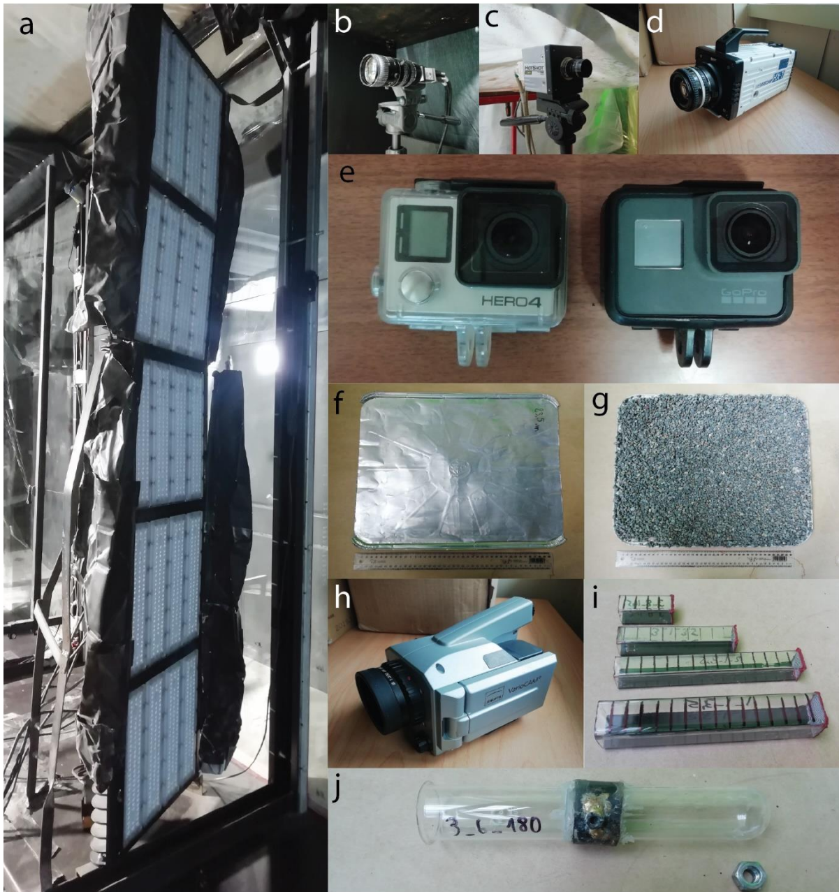
Figure 3.4: Material used for the experiments. a) LED flood lights tower located right before the start of the main window with the obstacles. (b, c, d) high-resolution, high-speed cameras. (e) two models of GoPro™ cameras. (f) deposit tray for the unconfined outside runout. (g) deposit tray of the confined interior channel, covered in glued bed roughness gravels. (h) thermal infrared camera used to measure temperature in the unconfined runout. (i) time-resolved square tube samplers of different size and width. They are graduated per centimetre and their downstream end is closed by layers of very fine mesh as described in Brosch and Lube (2020). (j) time-integrated tube sampler for bulk flow mass and grainsize distribution.
