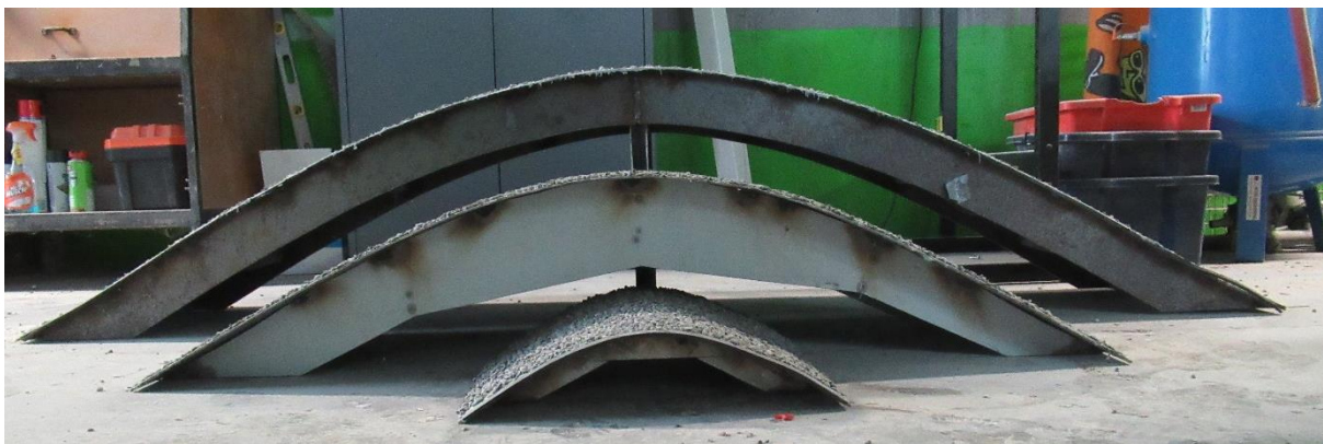
Figure 3.2: Photograph of the three obstacles. The smallest one is 10 cm high and 50 cm long, the intermediate one is 30 cm high and 1.5 m long while the largest one is 50 cm high and 2.5 meters long.
