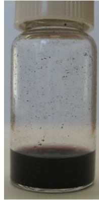
Figure 3.3 ppMWCNT suspension at 1mg/ml in FFM 10% three months after sonication. The suspension was relatively stable although a small amount of visible sediment accumulated on the bottom of the glass scintillation vial.
