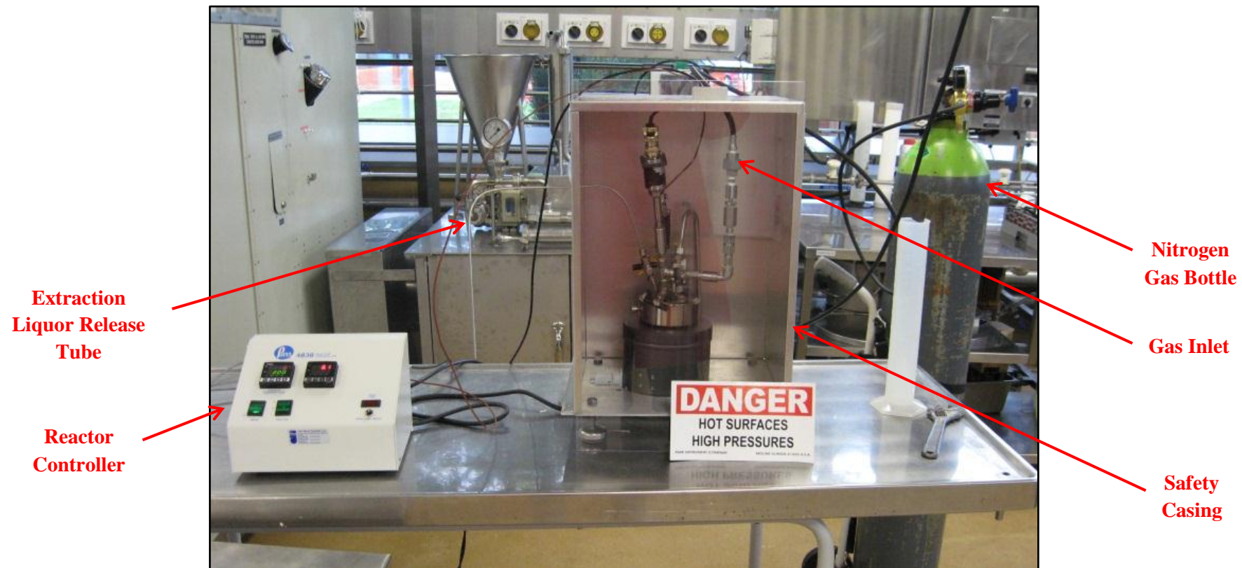
Figure 16. Final set-up of the Parr extraction vessel (quench water not shown).
