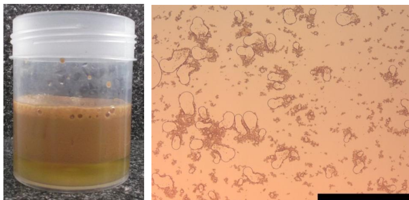
Figure H2. Photograph and LM image of a 20% (v/v) oil emulsion prepared using the fresh suspension method with 1.9% (w/v) lignin (bar scale = 500 \mu\text{m} ).
