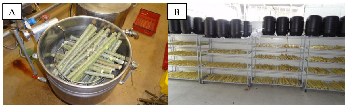
Figure C1. (A) Willow stakes loaded in steam jacketed vessel and (B) Storage of debarked stems on shelves (outside but undercover) for 2-3 days.
