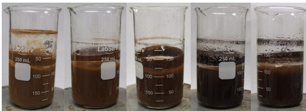
Figure 19. Photographs of microparticle suspensions prepared by shearing 30 mL of lignin extraction liquor into 75 mL water at temperatures of (from left to right) 4, 20, 40, 60 and 80°C.
