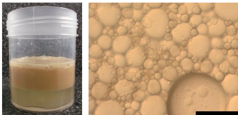
Figure H1. Photograph and LM image of a 20% (v/v) oil emulsion prepared using the pH-modification method with 0.1% (w/v) lignin (bar scale = 100 \mu\text{m} ).
