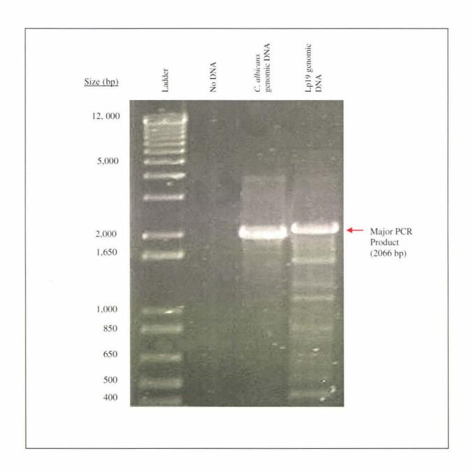
temperature of 54°C using 10 ng of template resulted in both a good yield of a product of the expected size (a 2035 bp product was expected using *C. albicans* DNA as a template, and a product of comparable size from Lp19 DNA) and low levels of other products for both *C. albicans* and Lp19 templates (Figure 3.2; section 2.2.9 using PCR protocol 7 (PR7) in Table A2.1)
