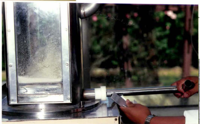
Figure 3.4. A close up view of the drying casein and the sampler in operation.
