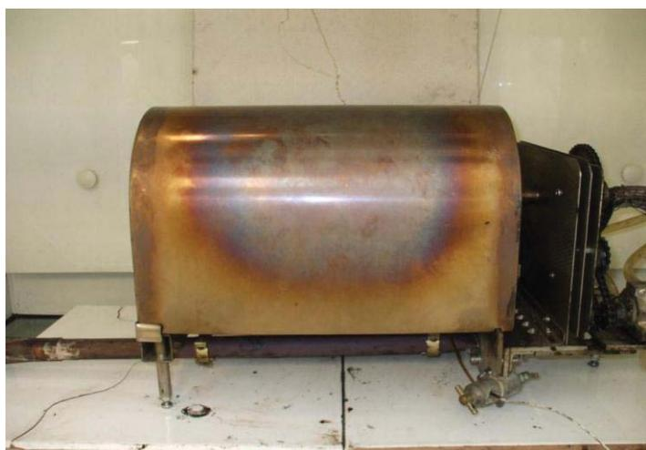
**Figure 2.1** Pyrolyser used for the manufacture of Biochar (Small, 5 L, rotating, gas fired cylinder)
