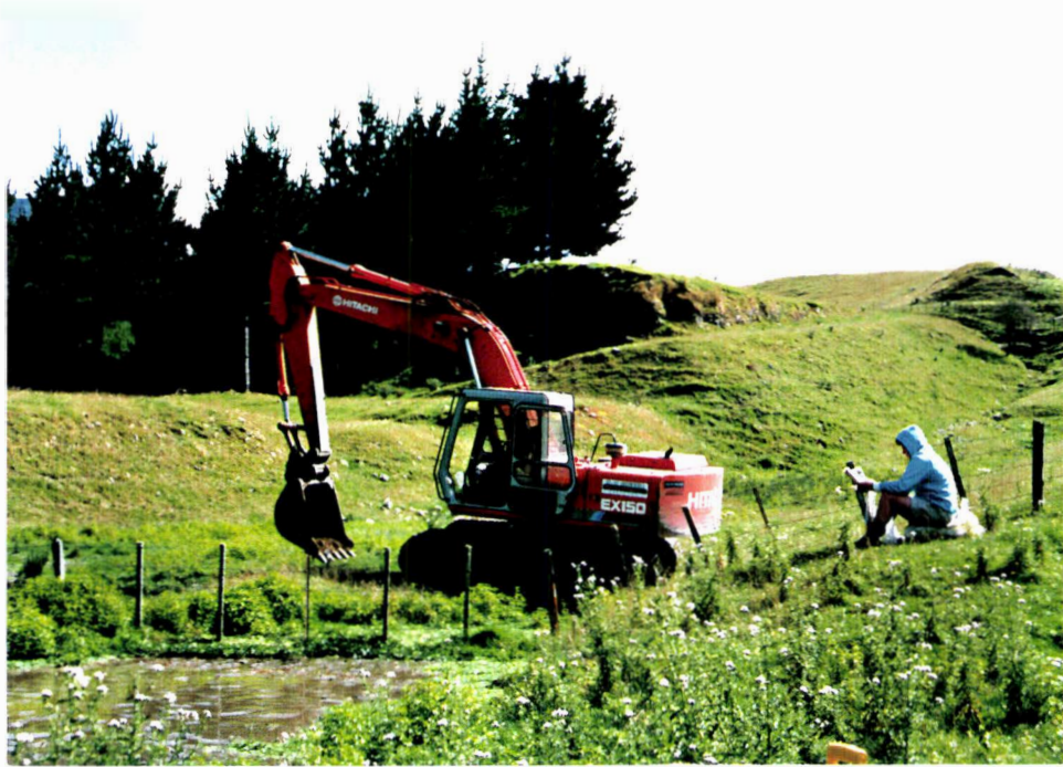
Plate 9, The Wellington Fault duplex at Inglis' farm. The Inglis 3 trench is being excavated. A farm track (f t) cuts the upthrown Ohakean gravels (Ohu) the two paleo-streams are behind the digger the oldest is marked (S1) and the younger (S2). Dr A S Palmer (Dept of Soil Science, Massey University) is seated on the downthrown Ohakean surface (Ohd).
