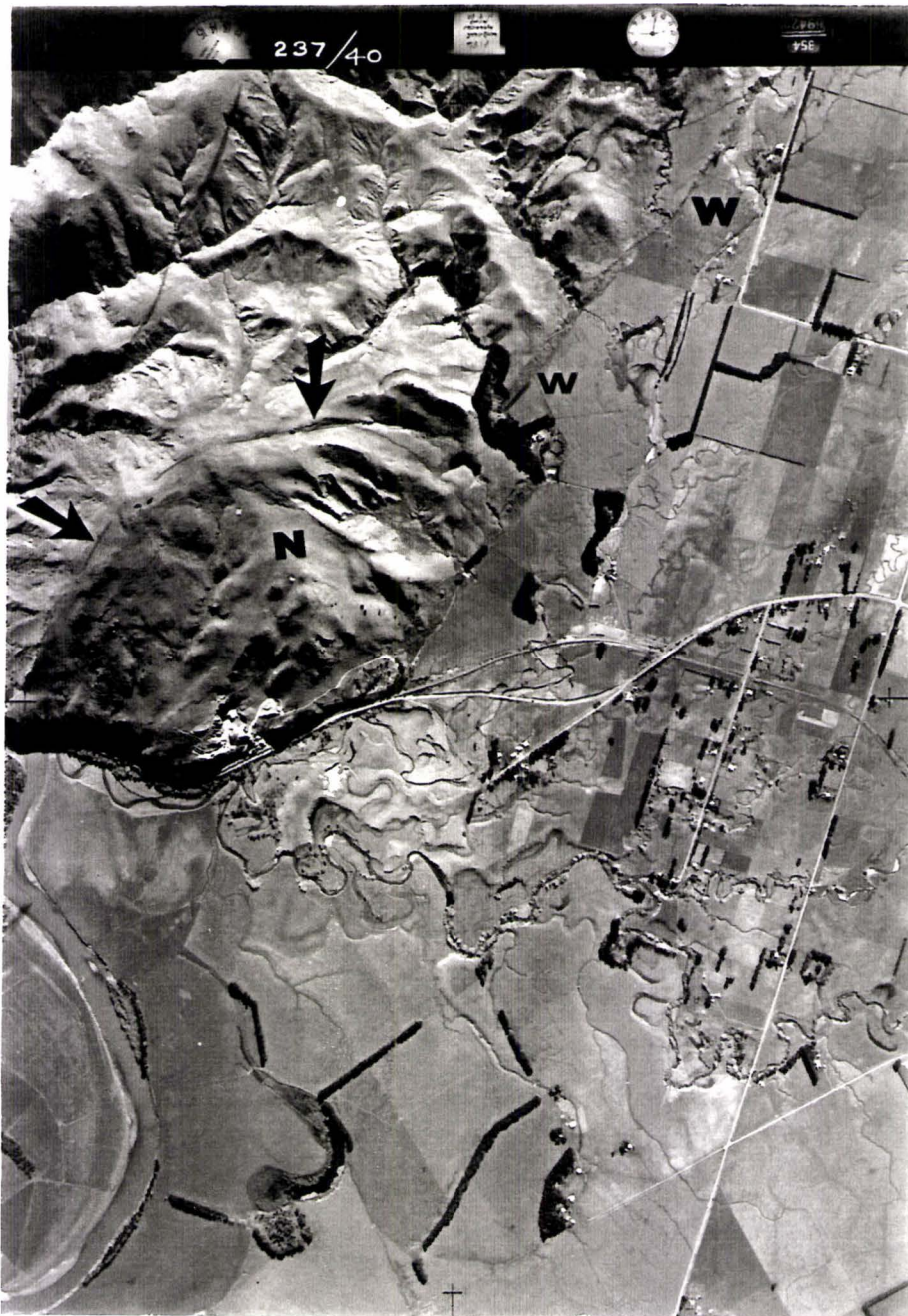
Plate 5, The stereo pair to Plate 4, showing the Nukumaruan limestone block (N) and the Wellington Fault scarp (W) to the north of the limestone. This scarp has been uplifted to the west between 15m and 19m close to the Ballantrae Research Station and offsets Ohakean terrace surfaces. The head scarp of the Nukumaruan limestone slump, is marked with arrows.
