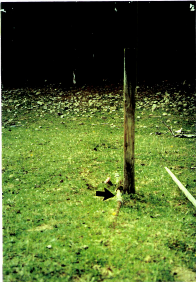
Plate 32, Above, Wellington Fault scarp at Gull Road, where a small amount of creep may be occurring along the fault trace. A galvanised pipe running at right angles across the fault scarp has been pulled apart twice since 1960. The pipe is (arrow) in the background.
