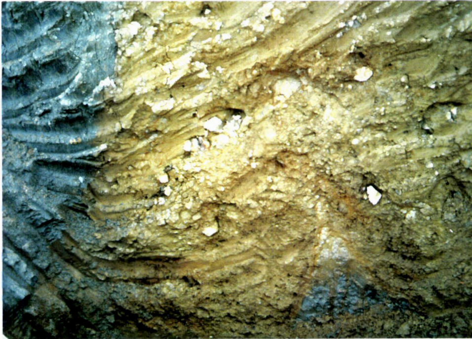
Plate 15, Inglis 4 trench north wall. The main fault plane (arrows) is visible where Tertiary mudstone (Tm) is upthrown 6m against younger Quaternary sediments to the east. This view also shows the listric fault (L) consisting of Tertiary mudstone with the overlying folded gravel units of pebbly (pg) and cobbly gravel (cg).
