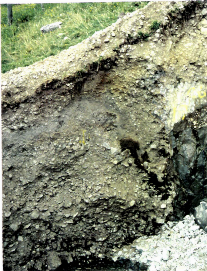
Plate 10, The main fault plane of the Wellington Fault as seen in the southwest wall of the Inglis 3 trench. The west wall of the fault is composed of Tertiary mudstone (Tm) which is overlain by Holocene gravels (H). Effects of subsequent deformation can be seen where finer (F) sediments have entered the gap between the bouldery gravels (bg) and the Tertiary mudstone in two consecutive episodes, labelled 1 and 2. Vertical displacement between 1 and 2 was measured at 0.9m
