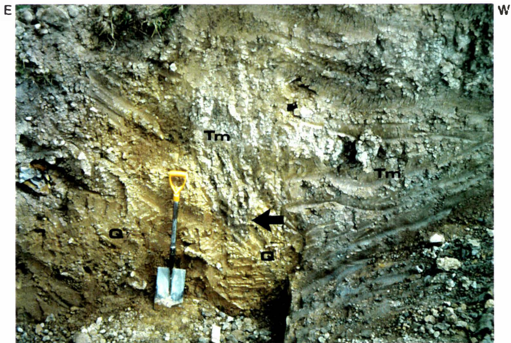
Plate 18, Inglis 4 trench, south wall showing a horse or slice of Tertiary mudstone (Tm) that has been thrust into Quaternary sediments (Q). The V section (arrow) was dug out with a pocket knife and has a bearing and plunge of 235/40^{\circ} which is 15^{\circ} oblique to the strike of main fault plane at this locality.
