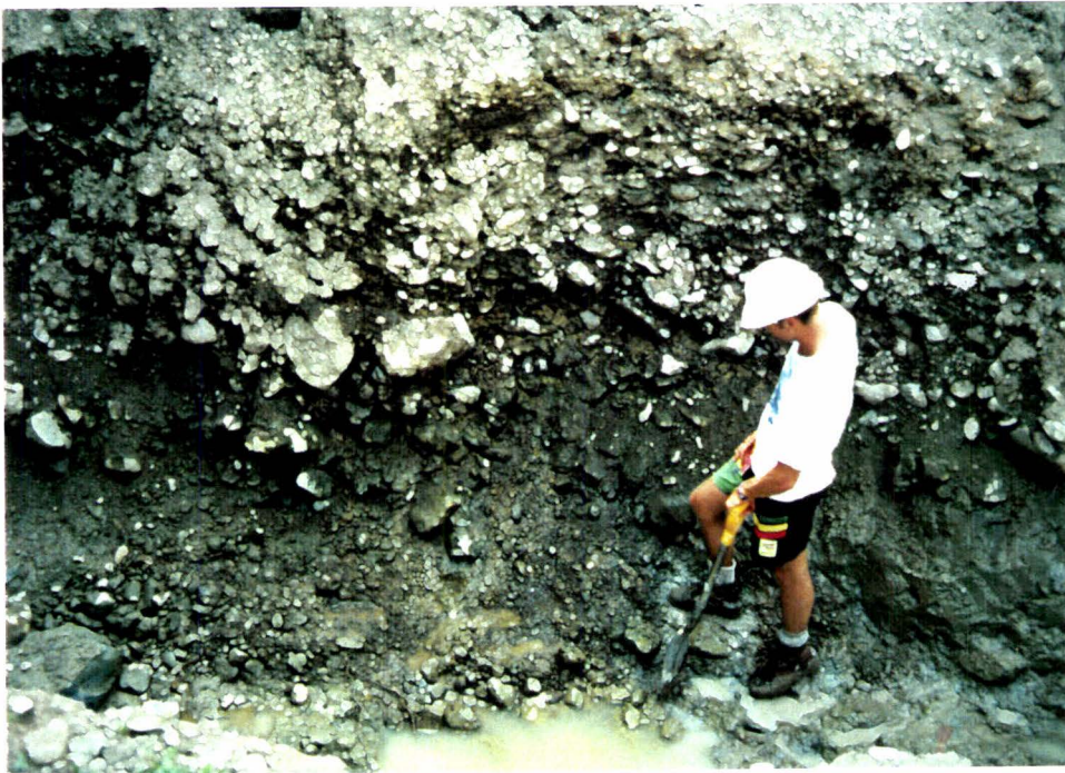
Plate 12, Wellington Fault, Inglis 3 trench northeast trench wall. This plate shows the east end of the mini-graben and the fault which created the graben (Figure 5). The unctuous clay (Uc) is vertically offset 0.9m. Some faint drag structures can be observed within the bouldery gravels (Bg). The second faulting episode in plate 10, has also been vertically offset 0.9m and is thought to have occurred at the same time as the above event.
