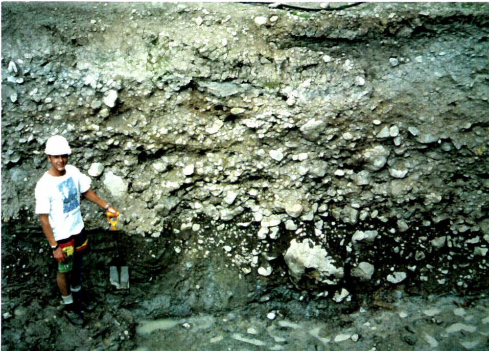
Plate 13, Inglis 3 trench excavated across the Wellington Fault, showing the south wall of the mini-graben and the fault which created this structure. The unctuous clay (Uc) is vertically offset 0.9m, some faint drag structures can be observed in the bouldery gravels (Bg). This deformation is thought to have occurred during faulting event 4 (Figure 8).
