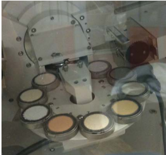
Figure 4-3 Samples loaded into the diffractometer for scanning
