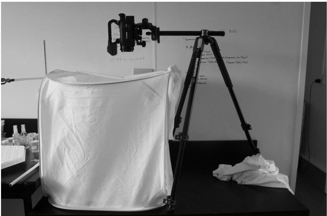
Figure 3.1. Laboratory assay set up. Assays were set up within mazes placed in a pop-up tent and recorded from above.
