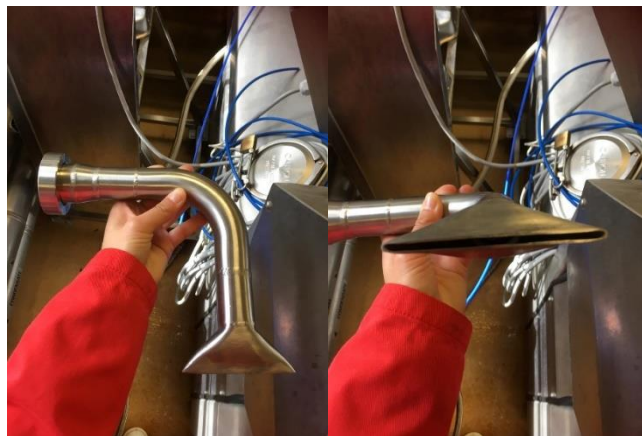
Figure 2.10. Extruder head attachment fabricated to fit the sausage stuffer
