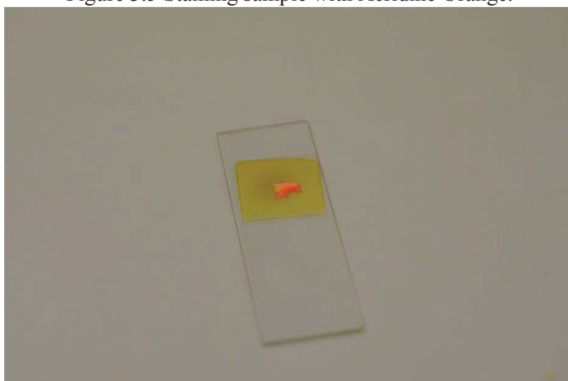
Figure 3.6 Coverslip on the top of sample with Nile Red (Invitrogen; 0.02% in methanol) and Acridine Orange (Riedel de Haen-Sigma Aldrich).
