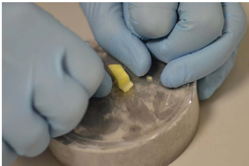
Figure 3.3 Shaving butter strip from a cube using 1.8 kg strength standard fishing tippet (Airflo-Hunting and Fishing NZ).
