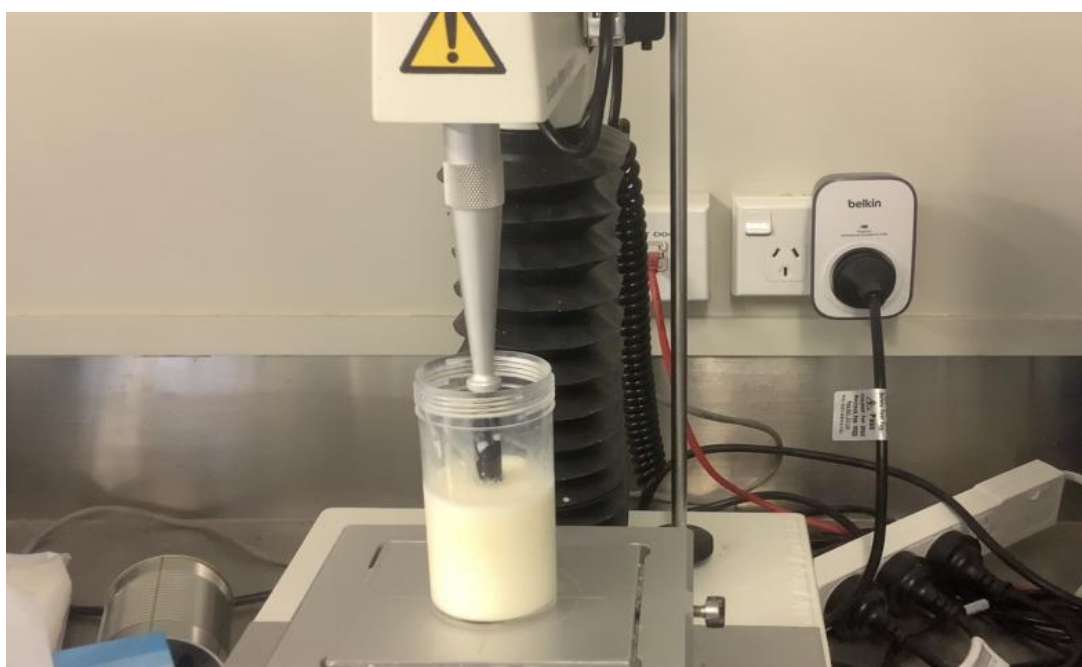
Figure 3.9 Setup for measuring the hardness of ice cream
