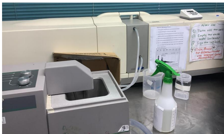
Figure 3.8 Setup for measuring the fat globule size distribution of ice cream mix and ice cream Images captured by iPhone 11, Apple Inc., California, USA.
