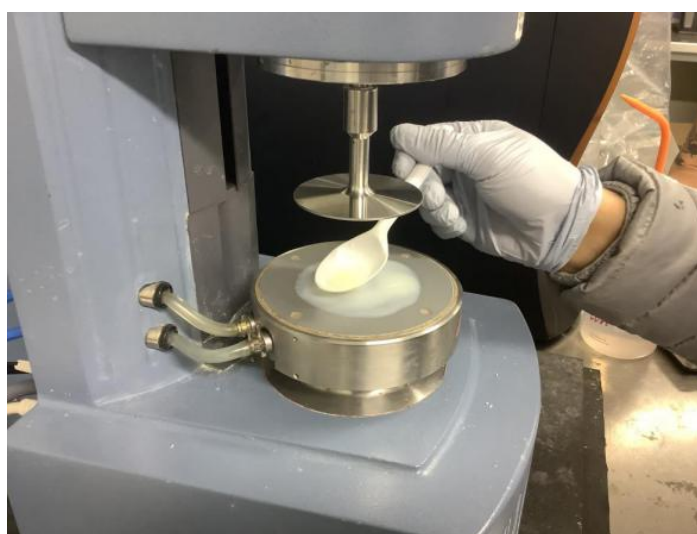
Figure 3.3 Setup for measuring the viscosity of sample Images captured by iPhone 11, Apple Inc., California, USA.
