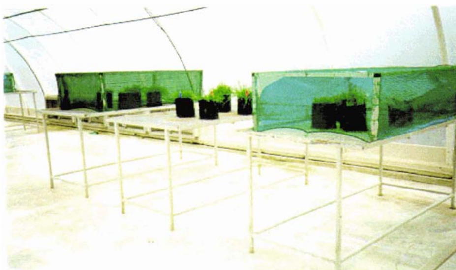
Figure 6.1 Experimental set-up showing one replication: 24% PAR plus reduced R:FR with the use of filters, and 25% PAR plus natural R:FR ,without filters.
