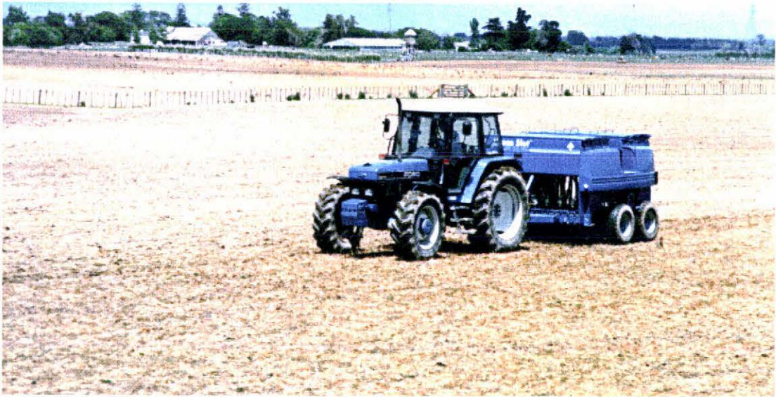
Figure 14: Cross-Slot™ no-tillage drill used for crop establishment.
