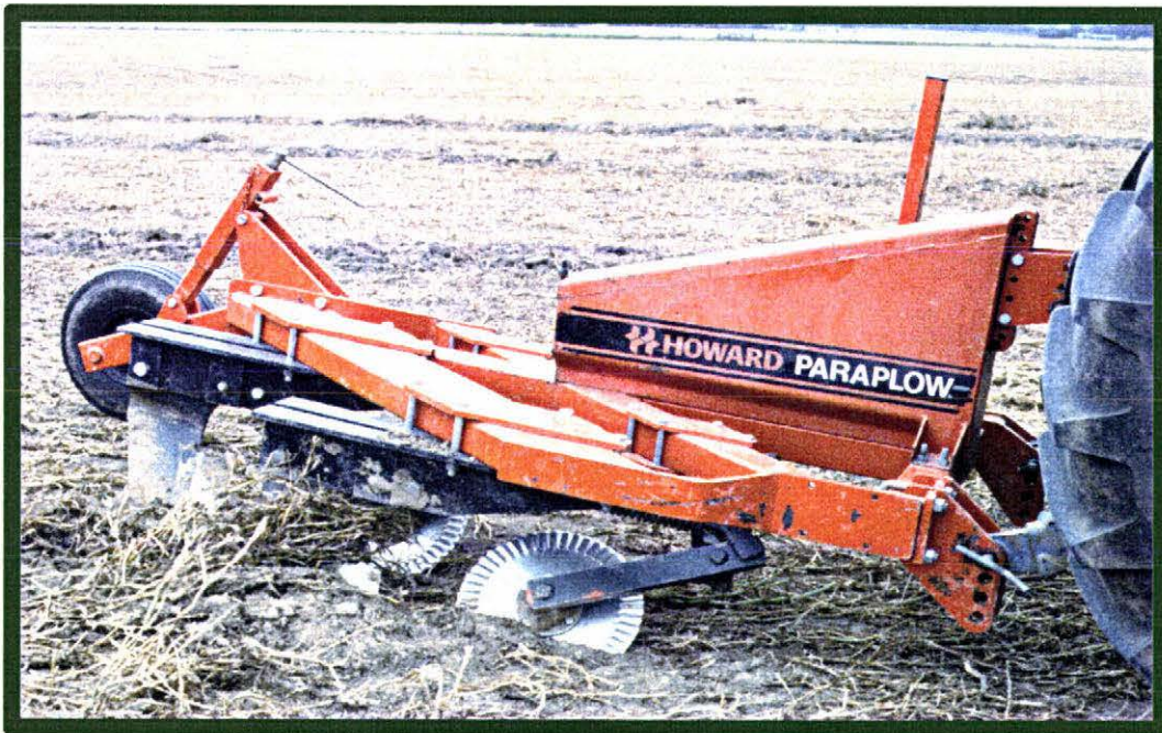
Figure 17: Howard two-legged Paraplow®.
