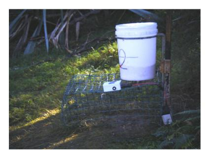
Plate 4. Feeder station set-up with data logger and antenna (Photo: J.Rickett)
