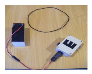
Plate 3. Data-logger, antenna and battery set-up (Photo: J.Rickett)
