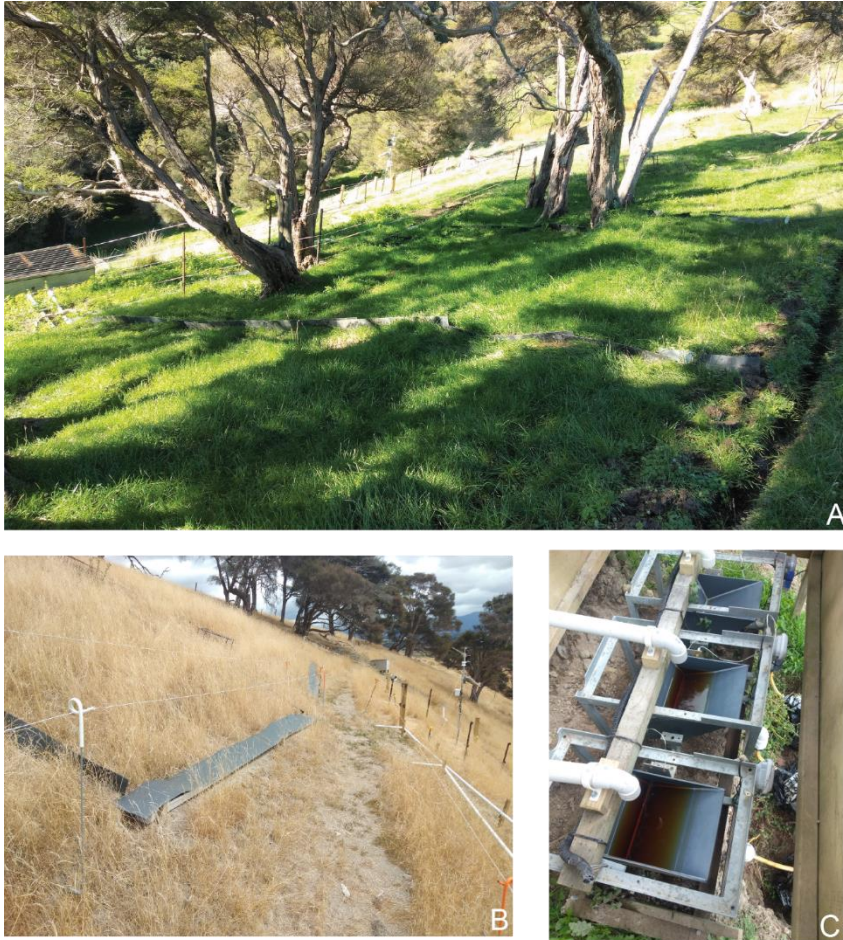
Figure 5.2. Surface runoff plot equipment. A: The kānuka pasture treatment plot 1–3 (the photograph was taken in early Spring). B: An open pasture plot (plot 5) and surface runoff collecting gutters covered by plastic edging (the photograph was taken in late summer, the pasture under kānuka became a similar colour in late summer). C: Tipping buckets collecting surface runoff. All photographs were taken by the lead author.
