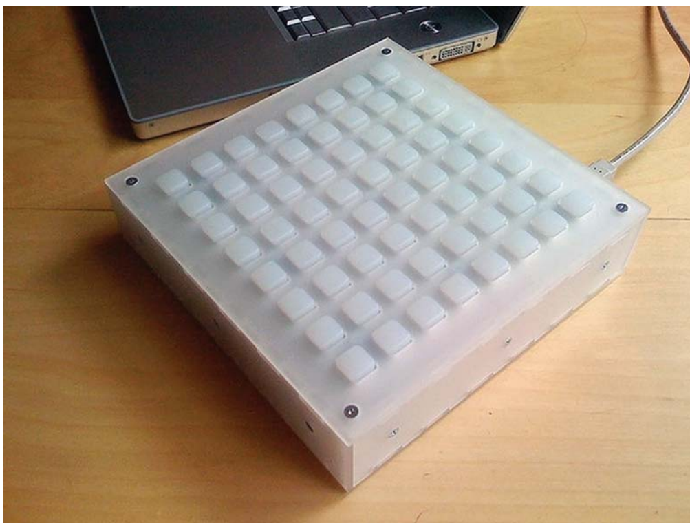
Figure 5: The first Arduinome. Built using Monome 40h buttons
