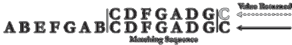
Figure 46: Matching sequences return the next stored state form the database
