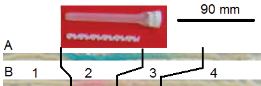
Figure 2.27 Output threads from a static mixer on adding 10 \mu\text{L} (A) or 1 \mu\text{L} (B) of concentrated food dye into a stream of idli batter. The static mixer barrel (90 mm with i.d. 8 mm and 4.5 mL volume) and the 10-element mixer insert (removed from barrel) are shown in the red box.
