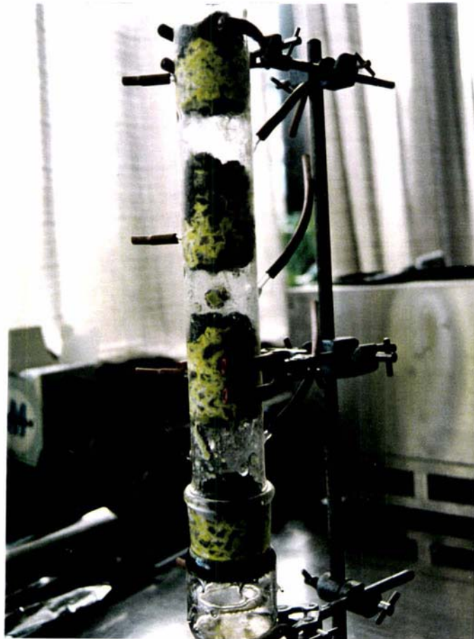
Figure 9.11 Morphological observation of the fermentation in a multi-layer packed bed reactor (5 days fermentation)
