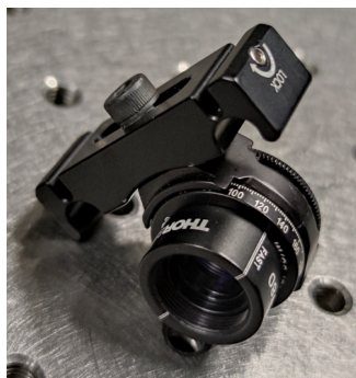
FIGURE A.7: A snap-on cage mount holding a half-inch rotation mount (see angle increments) and polarizing optic.
