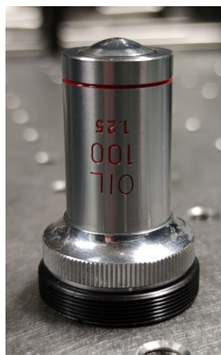
FIGURE A.6: The simple objective used for high-magnification Raman microscopy. Magnification = 100\times , NA = 1.25, f \approx 1.66 mm, clear aperture D \approx 5 mm.
