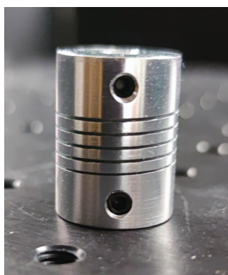
FIGURE A.8: A flexible mechanical coupling for mitigating run-out issues. Not used in the final designs due to backlash and hysteresis issues.
