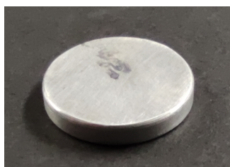
FIGURE A.9: An aluminium disc used for loading samples in the LT Linkam stage. The dark spot in the image is some MoS 2 powder pressed into the metal.
