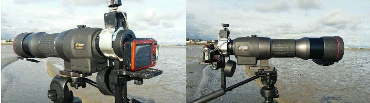
Figure 3: Nikon scope and camera mount setup for use in the field.
