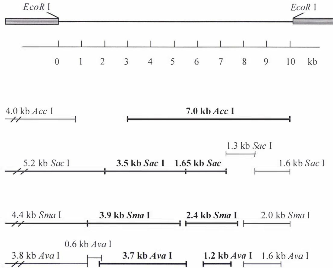
**Figure 18:** Third group of restriction digests of the 10 kb *EcoR* I subclone
