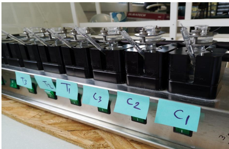
Figure 4.4: Multi-station Franz diffusion cell system used for in vitro permeation study
