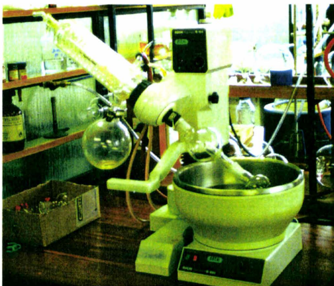
Fig 2.10 The rotary vacuum flask used to remove the ether from the reaction products.
