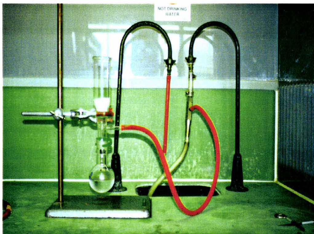
Fig 2.9 The celite filter used to remove the \text{PtO}_2 catalyst.
