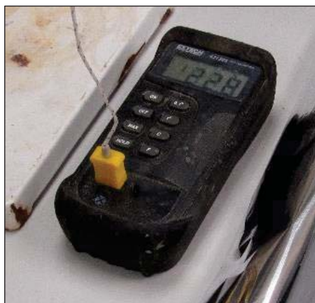
Figure 8: The thermocouple used in monitoring the temperatures of the water dripping into the Soxhlet reactor holding the volcanic ash sample.
