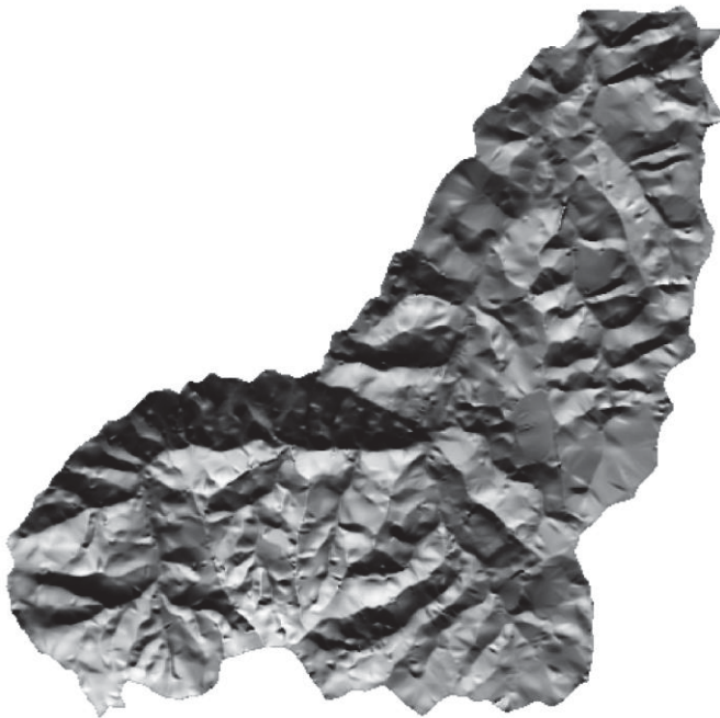
Figure 10. Relative solar radiation map for July. Darker shades are lower values (relatively less radiation). Minimum value = 0.025. Maximum value = 1.79.
