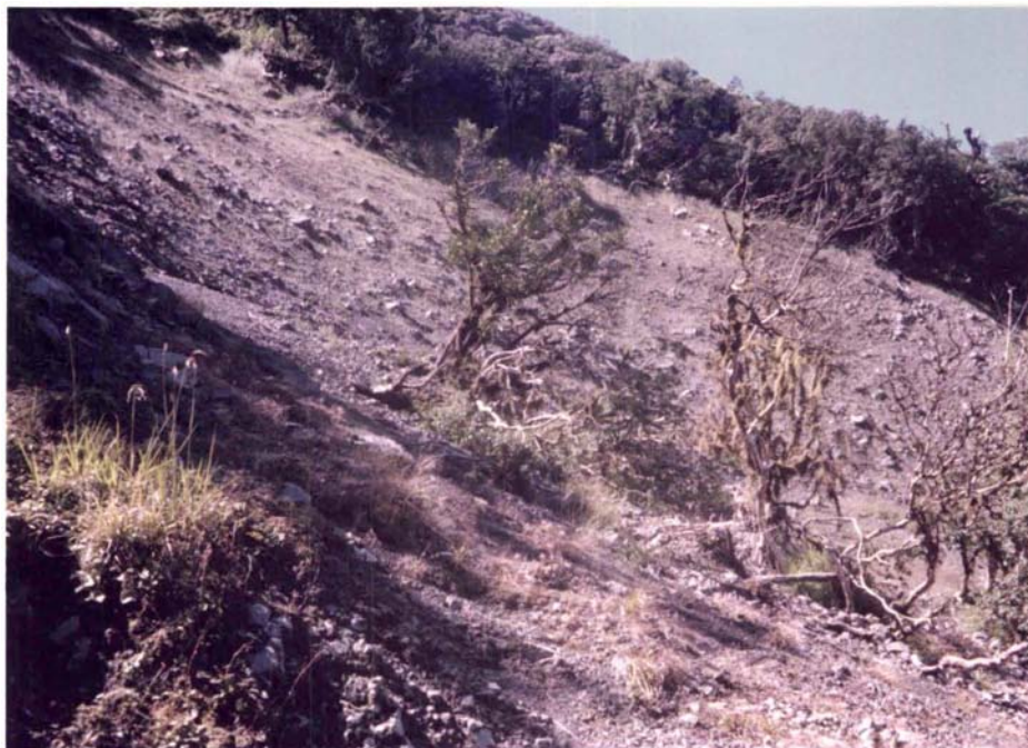
FIGURE 10.2: Close-up of debris slide scar within Mangapuaka catchment. Note: (1) the shallow depth of failure (less than 0.5m) within colluvial slope material; (2) the dense shrubby vegetation (background) adjacent to where the movement occurred; and (3) the shallow root systems of the vegetation on the slide (foreground).
