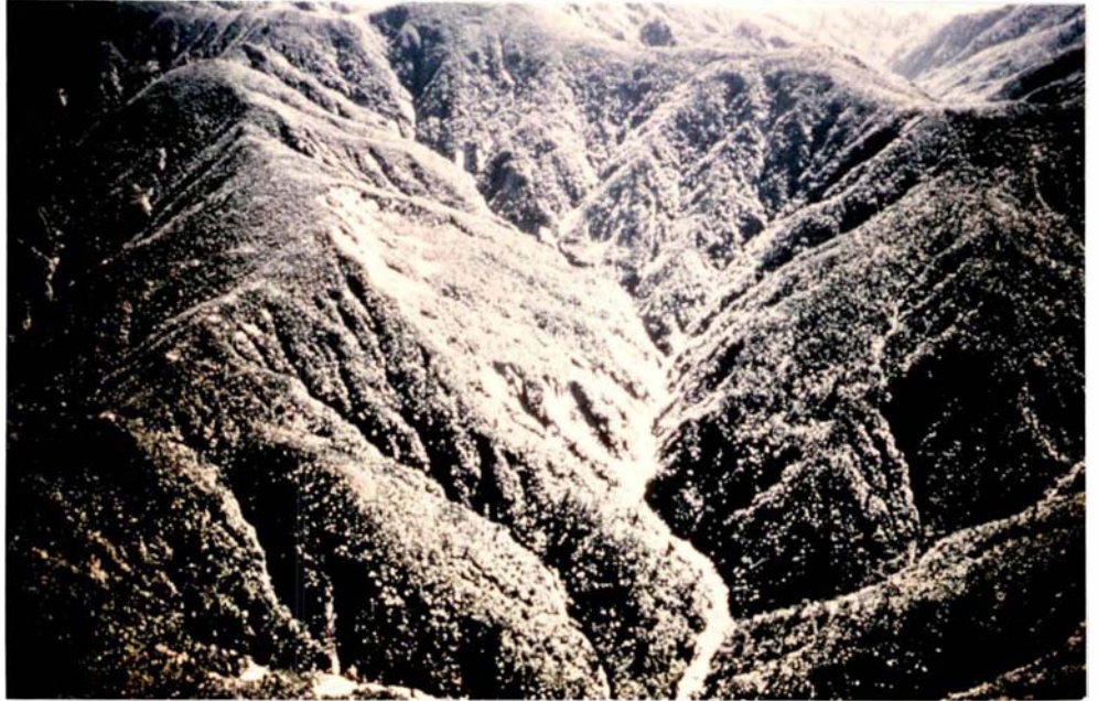
FIGURE 10.17: Large-scale rock slump with well defined lateral and head-wall scarps. Slump movement is towards the north (right). This slump sits astride a 500m wide, northeast striking fault breccia zone mapped as the Ruahine Fault. Note the occurrence of debris slides in the headwall area and gully erosion together with debris slides in the toe area of the slump, much of which has developed since 1946 (see Chapter 11).
