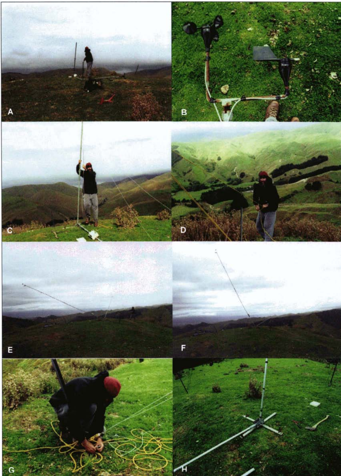
Figure 7.3 The systematic anemometer mast raising technique including details of the mast assembly.
