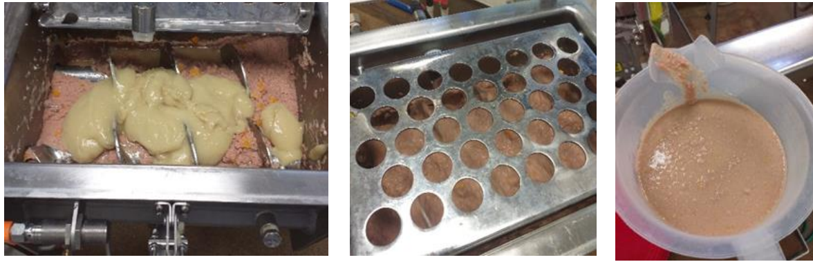
Figure 5-4: Addition of thick emulsion to Blentech by opening grate.
