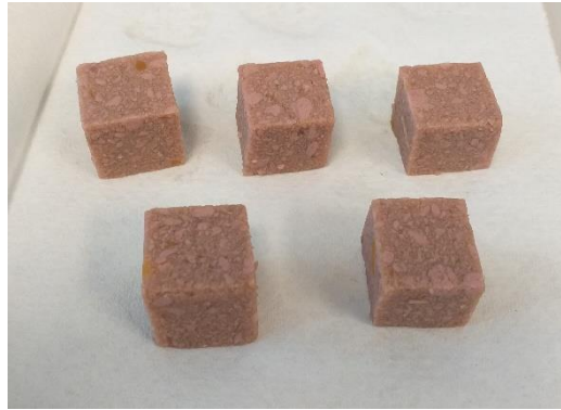
Figure 3-3: Test samples for TPA analysis prepared using a double-edged knife to obtain cubes approximately 2 cm 3 .
