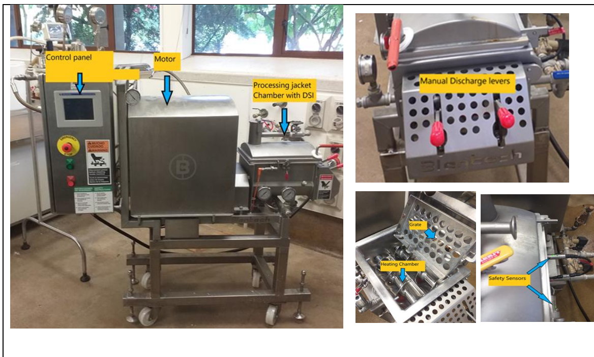
Figure 4-2: The Blentech CC10 Steam injected pasteuriser.
