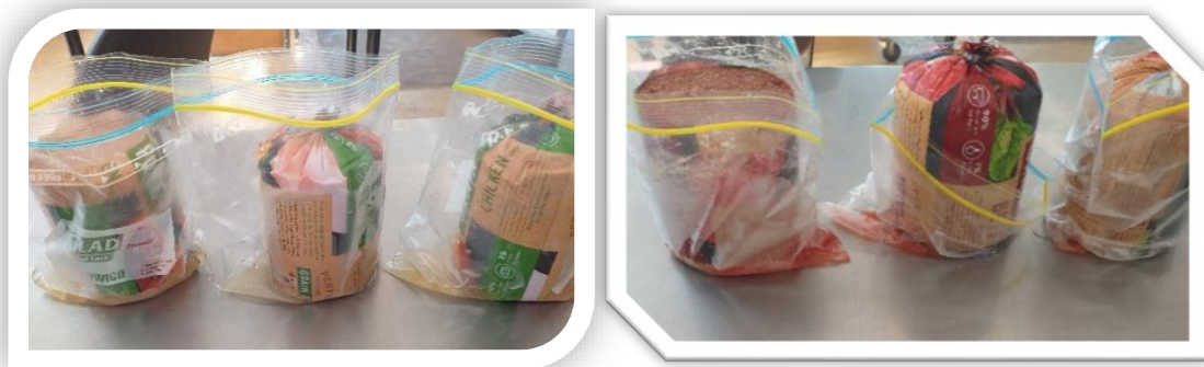
Figure 3-6: Factory roll samples exhibiting thaw drip loss after the freeze thaw treatments.
