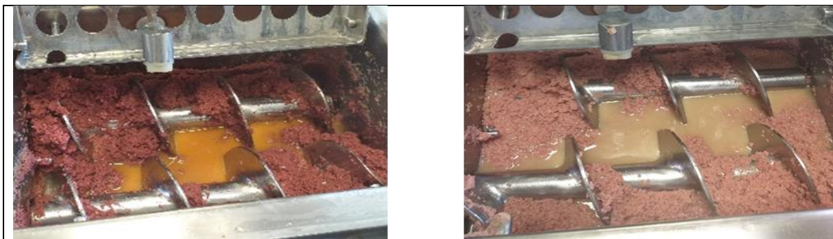
Figure 5-10: New Beef (left) and Chicken meat (right) after processing @ 85 °C for 15 minutes.
