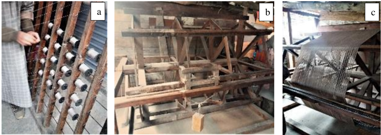
Figure 4.14 A Kross containing yarn rolls (a), a wooden wheel for transferring the yarn rolls from the Kross (b), yarn transferred from the Kross onto the wooden wheel (c)
