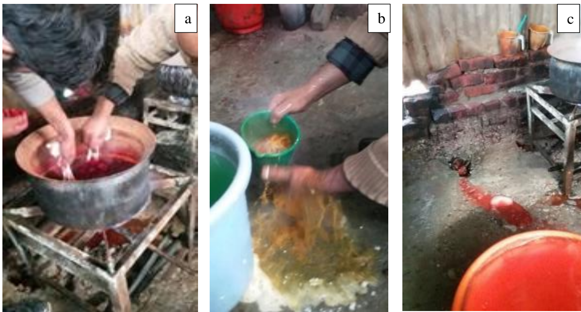
Figure 5.1 The dyeing process involves colouring the yarn (a), discharging the water in the drain (b) and washing of hands post completing the process (c)
