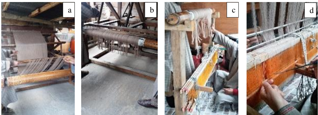
Figure 4.15 Yarn is being lifted from the wheel (a), yarn is being transferred on to a cylindrical log (b), yarn is being shifted from the cylindrical log (c), yarn is being arranged in a specific pattern for weaving on a handloom (d)
