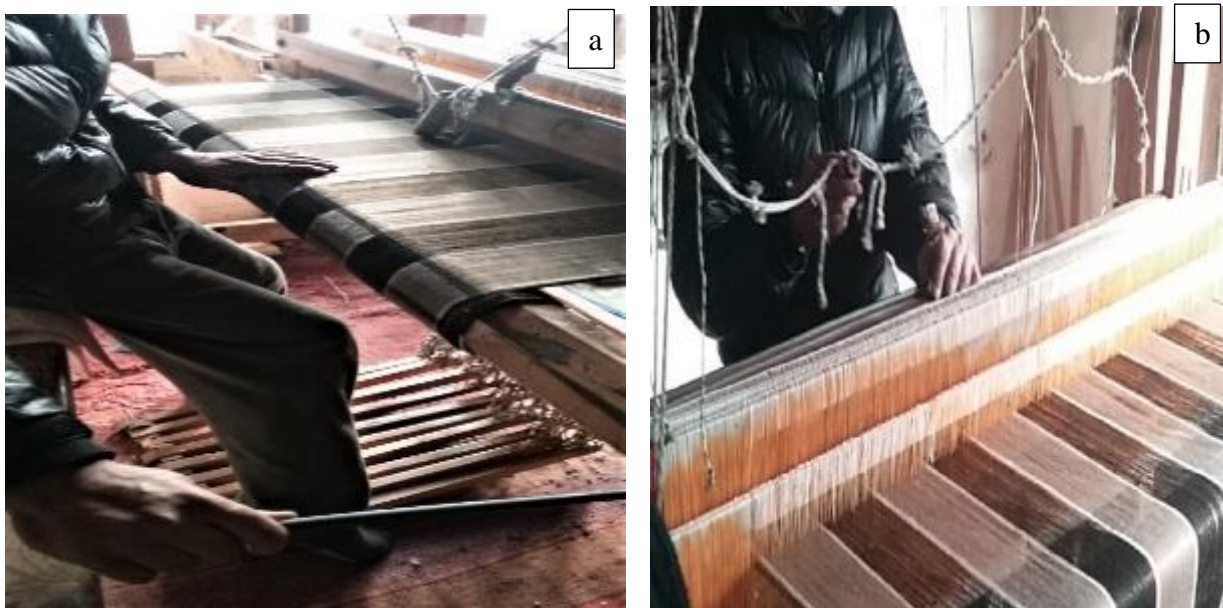
Figure 4.16 Foot pedals in a handloom (a), a weaver working on an advanced handloom (b)
