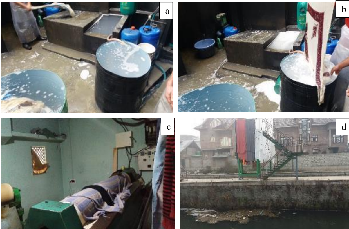
Figure 4.22 A washerman striking the fabric on a cement platform (a), a shawl being washed by a washerman (b), rolling iron press to dry the fabric (c), fabric being sun dried (d)
