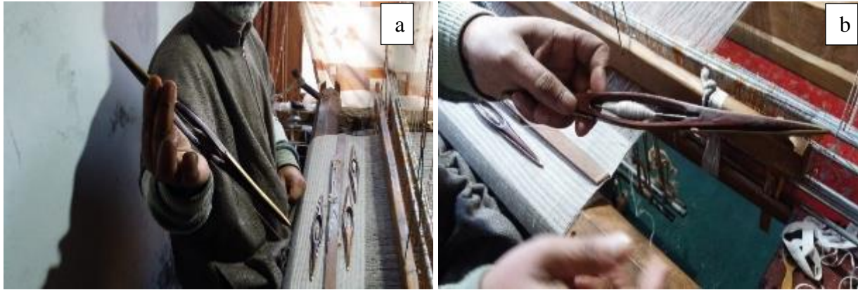
Figure 4.17 A weaver working on a traditional handloom showing the Muk (a), a closer look of the Muk (b)
