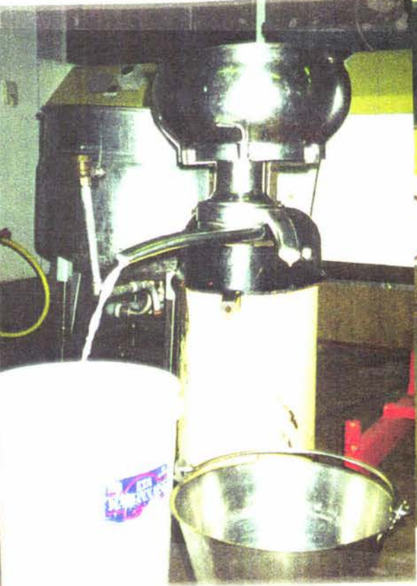
P2: Skimming: Centrifugal separator
