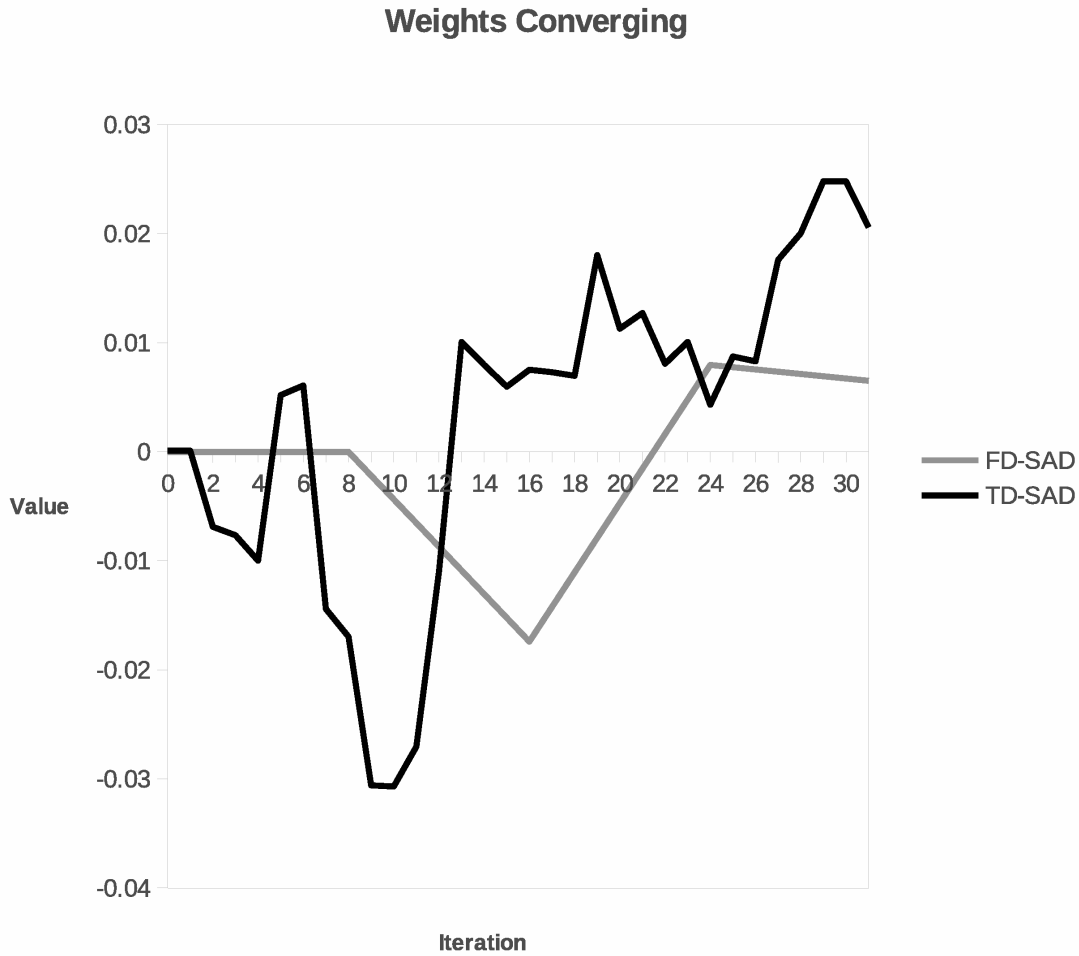
Fig. 5.4: The convergence of the tap at index one over 32 time samples when \mu = 0.2 .
