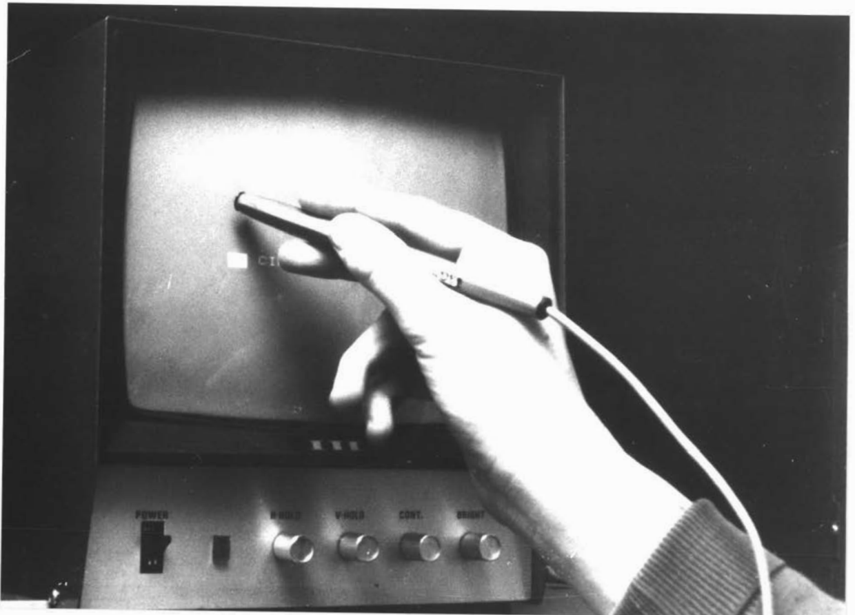
Responses can be input to the computer using a light sensitive pen.
