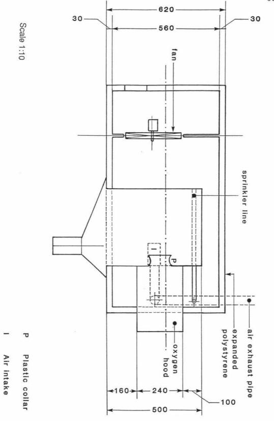
FIGURE 2: SIDE ELEVATION OF CLIMATE CHAMBER
