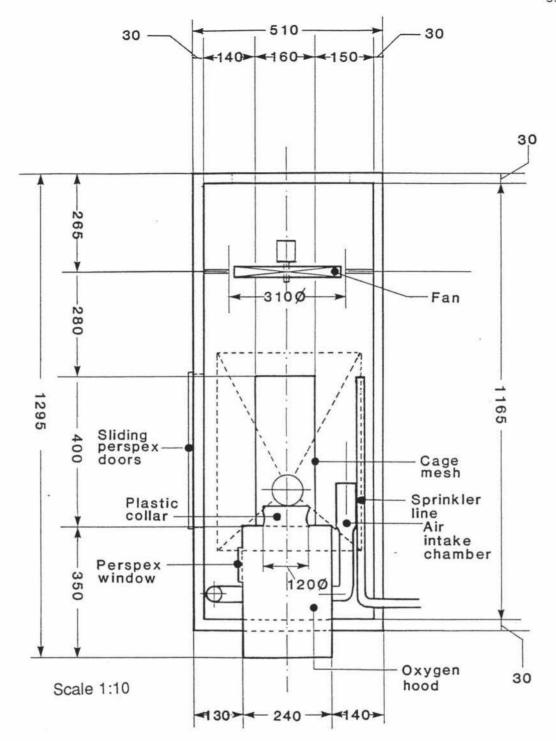
Figure 1: PLAN VIEW OF CLIMATE CHAMBER
