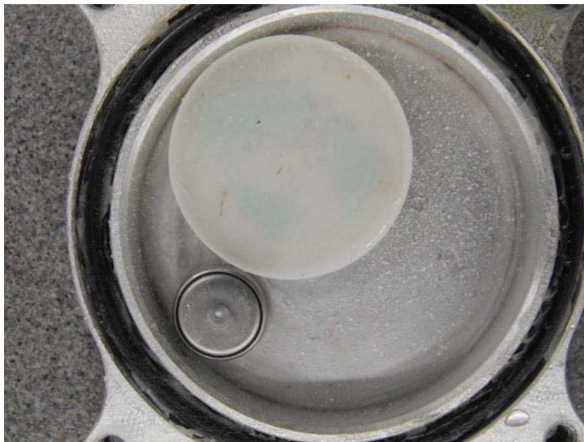
Figure 3-11: Sample pan with saturated salt solution and ibutton (bottom).
