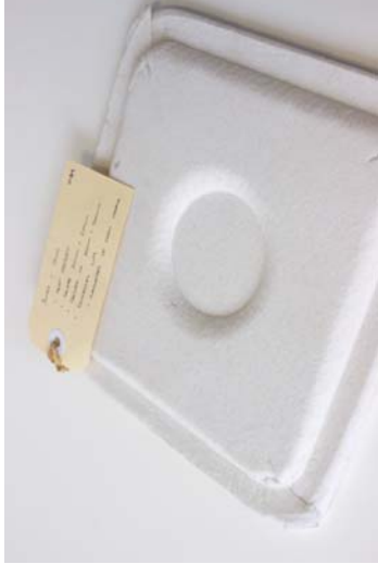
Figure 87 Material: Autex Cube™ 12mm. Test: Heat pressing. Aim: Controlled shaping of the panel product. Results: Crisp details exposed in moulding. The oversize panel shrank slightly when heated to fit the cavity. Edges were cut and overlapped to fit into the radius. Process is zero waste.
