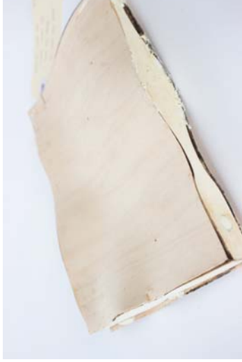
Figure 128 Material: Oak veneer / Expanding foam. Test: Making lightweight, complex-surfaced timber panels. Aim: Exploring possibilities of veneer composites. Results: The new composite material is lightweight and strong. The foam provides some sponginess. Process is not zero waste because of the border frame.
