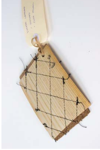
Figure 44 Material: Oak veneer / Cotton thread / Cork. Test: Stitched laminate with substrate. Aim: Added cushion to laminate. Results: Aesthetic lamination technique, less spongy than cardboard. Process is zero waste.
