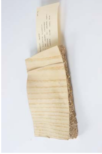
Figure 160 Material: Ecovative mycelium sample / Ash veneer. Test: Mycelium compound surfaced laminate. Aim: Increasing strength properties of mycelium. Results: The veneer layer provides great strength improvements while maintaining the materials flexibility.
