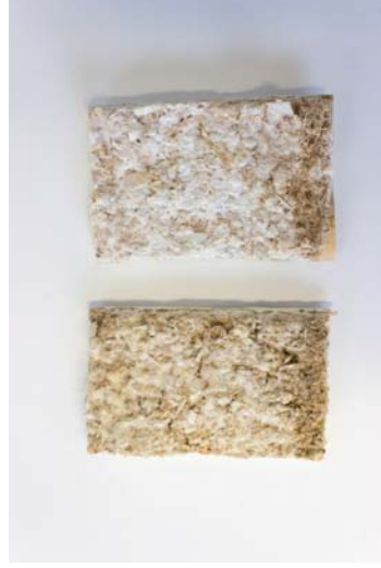
Figure 246 An experiment comparing the drying of the mycelium block in an oven vs. in the open air. The left block was left in an oven at 60° Celsius for 6 hours. The right block was dried outdoors in the sun for one week.
