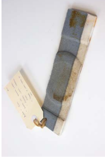
Figure 79 Material: Autex Workstation 6mm. Test: Boiling water forming using press. Aim: Controlled shaping of the panel product. Results: Autex is pliable when its exposed to boiling water. When pressed, the density of the Autex panel increases, improving its strength. Process is zero waste.
