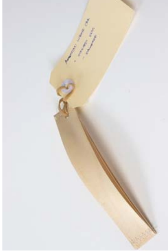
Figure 100 Material: Timber veneer / Cotton thread. Test: Stitched together three veneer sheets while bent. Aim: Stitch veneer into a complex form. Results: Exaggerated bending of sheets creates tension on those beneath, holding the form in an arc. Process is zero waste.
