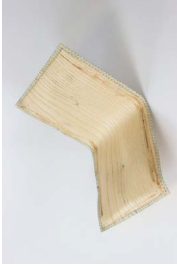
Figure 144 Material: Ash veneer / Cotton thread / Expanding foam. Test: Stitch detailing as a functional design consideration. Aim: Seal the veneer edges with a glue-less method while cavity is filled with expanding foam. Results: No expanding foam leaked out through the stitched edging. The coloured thread provides an aesthetic detail.
