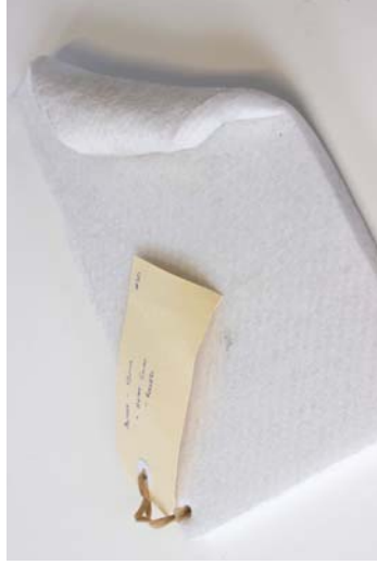
Figure 74 Material: Autex CubeTM 12mm. Test: Heat rolled. Aim: Controlled shaping of the panel product. Results: Autex is pliable when heat is applied. Once the plastic cools down, it forms to the new shape. Process is zero waste.
