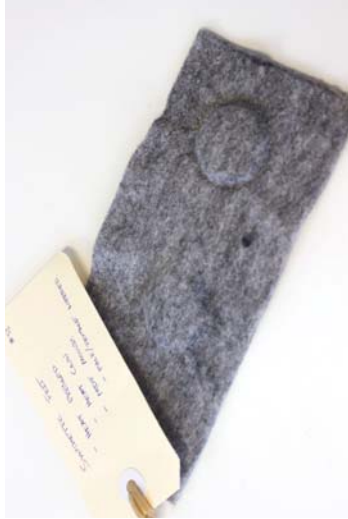
Figure 71 Material: Synthetic felt. Test: Heat pressed with positive and negative mould. Aim: Adding structure and value to textiles. Results: Felt doesn't stretch very much even with heat. The moulded form didn't add structure to the material. Process is zero waste.
