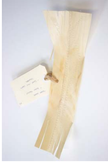
Figure 94 Material: Timber veneer / Cotton thread. Test: Stitched together two veneer sheets. Aim: Alternative material joining technique. Results: Aesthetic joining technique. Process is zero waste.
