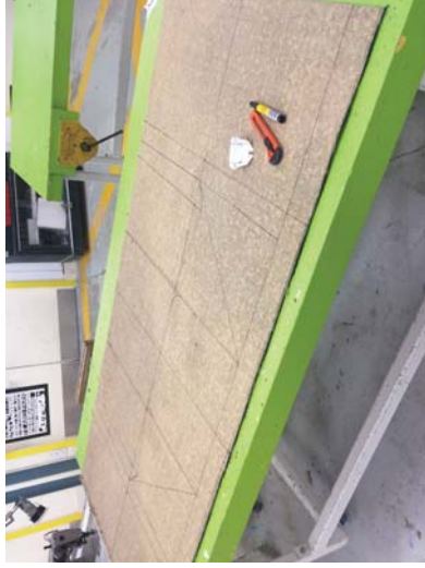
Figure 183 Zero waste pattern making on a strip of wool carpet.
