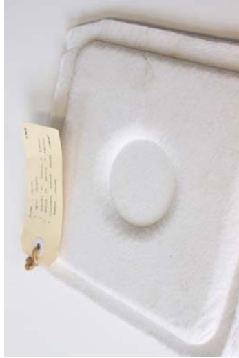
Figure 86 Material: Autex Cube™ 12mm. Test: Heat pressing. Aim: Controlled shaping of the panel product. Results: Crisp details exposed in moulding. The oversize panel shrank slightly when heated to fit the cavity. Edges were pushed into form the radius. Process is zero waste.
