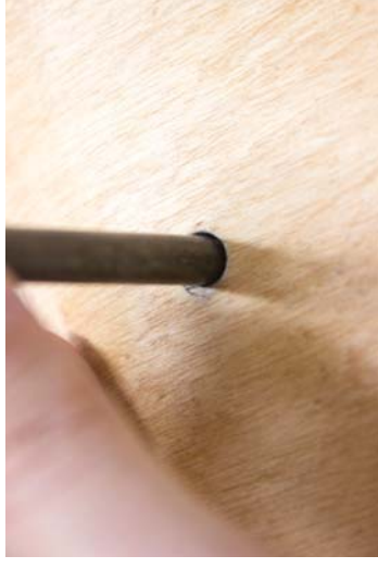
Figure 346 Punching veneer into the mycellium below.
