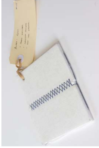
Figure 83 Material: Autex Workstation 6mm / Cotton thread. Test: Stitch joint. Aim: Joining two sheets of Autex with zero waste. Results: A flexible joint was achieved using a cross stitch pattern. Process is zero waste.
