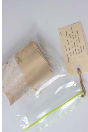
Figure 153 Material: Mycelium / Pine wood waste / Oak veneer. Test: Finishing mycelium samples. Aim: Exploring possibilities of growing material laminates. Results: The surface mycelium is easily removed using sandpaper. The natural timber can be finished using traditional means.
