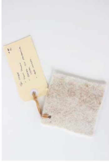
Figure 120 Material: Polyester fibre. Test: Felted in industrial felting machine, then heat pressed. Aim: Add structure and rigidity to polyester fibre. Results: Felting polyester fibre meshes the fibres together. Its textile structure increases when heat pressed. Process is zero waste.
