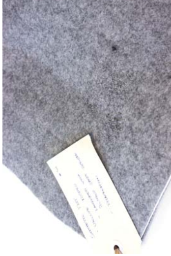
Figure 72 Material: Synthetic felt / Polypropylene sheet. Test: Vacuum formed with centre layer of thermo-plastic. Aim: Adding structure and value to textiles. Results: Felt doesn't stretch very much even with heat. The layers didn't fuse together well. Delamination occurred. Process is zero waste.
