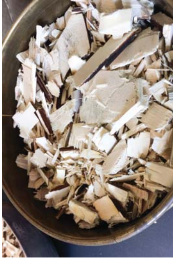
Figure 252 Separating the different sizes of wood chips for use in my mycelium samples. Mycelium works best when there is a variety of matter to feed on. The smaller pieces make a denser block, but larger pieces make it stronger.
