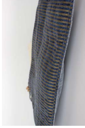
Figure 231 Expanding foam textile composite – expanded inside a fabric pillow. The resultant form looks soft but is quite firm.
