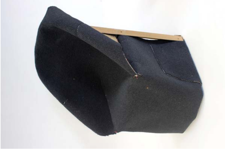
Figure 185 Second development of the carpet chair. The pattern was extended to incorporate legs. Extra bracing was required to support the structure of the chair; without it, it is not able to support its own weight.
