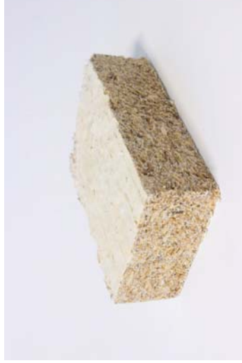
Figure 154 Material: Ecovative mycelium sample. Test: Sample material. Aim: Testing strength properties. Results: The white surface layer of the Ecovative mycelium is durable. The substrate is crumbly once exposed from the cut.
