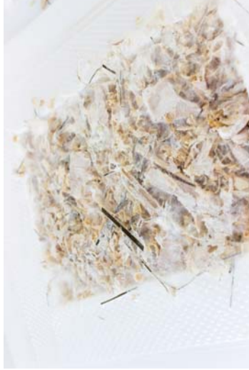
Figure 249 Mycelium sample grown in wood waste and flax fibre. The mycelium did not grow as dense in these samples. The anti-fungal properties of the flax slowed its growth.
