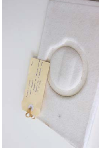
Figure 81 Material: Autex Cube™ 12mm. Test: Heat pressing. Aim: Controlled shaping of the panel product. Results: A form was pressed into the 12mm panel to 6mm, improving its rigidity. Process is zero waste.
