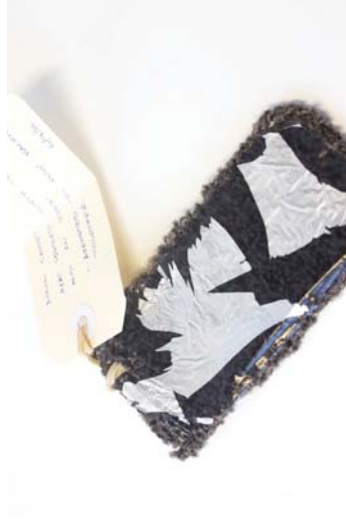
Figure 49 Material: Nylon carpet. Test: Heat pressed using iron and tinfoil / heat folding. Aim: Adding structure and value to carpet waste. Results: Surface aesthetics change, little structure is added. Nylon not fully melted through. Tinfoil fuses to the melted carpet and if difficult to pull off. Process is zero waste.
