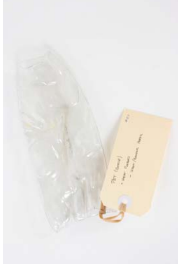
Figure 125 Material: PET plastic bottle. Test: Heat pressed using iron and baking paper. Aim: Adding structure and value to plastic waste. Results: Plastic did not press completely flat. The material shrank when heat was applied.
