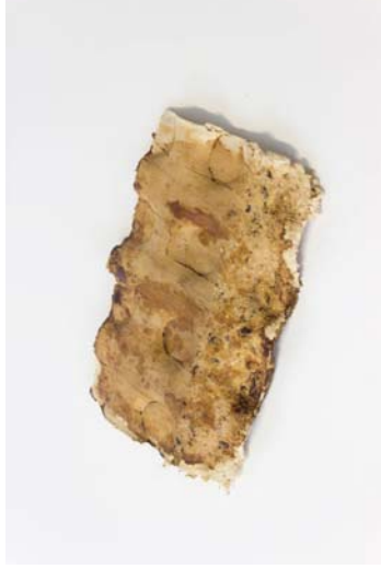
Figure 140 Material: Mycelium / Ash wood waste / Oak veneer. Test: Making a lightweight, natural composite material. Aim: Exploring possibilities of growing materials. Results: The new composite material is lightweight. Once grown with the veneer, the sample was pressed into a dense board.
