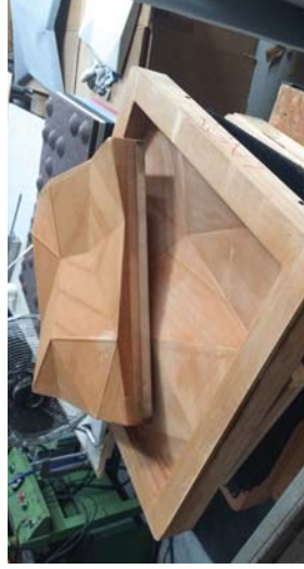
Figure 192 The two-part MDF mould for the Autex wall paneling. The mould is coated with a resin to harden the surface for repetitive use.
