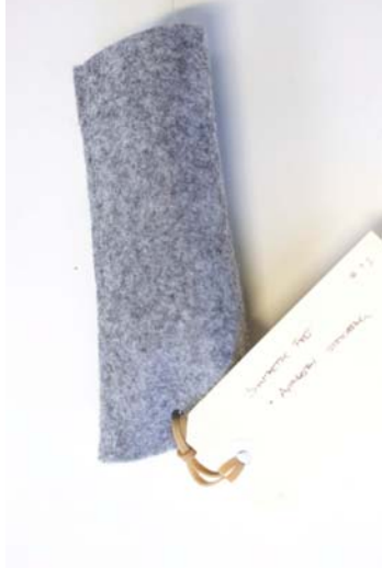
Figure 111 Material: Synthetic felt / Cotton thread. Test: Upholstery stitching felt into a cylinder. Aim: See what kinds of structure can be obtained with felt. Results: Because the stitching is done inside out, the cylinder must be reversible to look correct. Process is zero waste.
