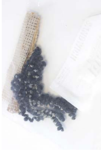
Figure 62 Material: Wool carpet. Test: Carpet deconstruction. Aim: Exposing alternative functions of wool carpet. Results: Wool carpet is far easier to deconstruct than synthetic carpet. The fibres pull out into a continuous yarn. Latex is fused with the yarn rather than the backing.
