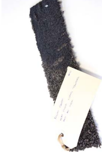
Figure 48 Material: Nylon carpet. Test: Heat pressed using iron and tinfoil. Aim: Adding structure and value to carpet waste. Results: Surface aesthetics change, little structure is added. Nylon not fully melted through. Tinfoil fuses to the melted carpet and is difficult to pull off. Process is zero waste.
