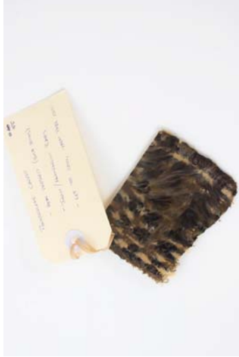
Figure 124 Material: Polypropylene carpet. Test: Heat pressed using iron and aluminum plates. Aim: Adding structure and value to waste carpet. Results: Polypropylene has a much lower melting point than nylon. When overheated, the carpet pattern starts to morph. Process is zero waste.
