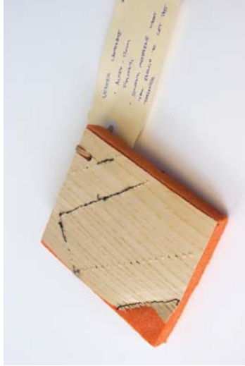
Figure 47 Material: Oak veneer / Cotton thread / Autex Cube™ 12mm. Test: Stitched laminate with substrate. Aim: Added cushion to laminate. Results: Aesthetic lamination technique. The substrate was too thick to sew successfully. Process is zero waste, but is not recyclable or decomposable as a composite.
