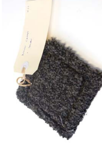
Figure 101 Material: Nylon Carpet / Cotton thread. Test: Zigzag stitch. Aim: See what effects can be made using a sewing machine. Results: The carpet fibres engulf the stitching details.
