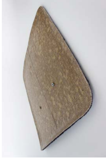
Figure 187 Moulding wool carpet with epoxy resin in a vacuum bag. The scaled up experiment is to understand how the composite functions as a seat base. A seat base must support a person's body weight, plus extra forces when sitting down and changing postures.
