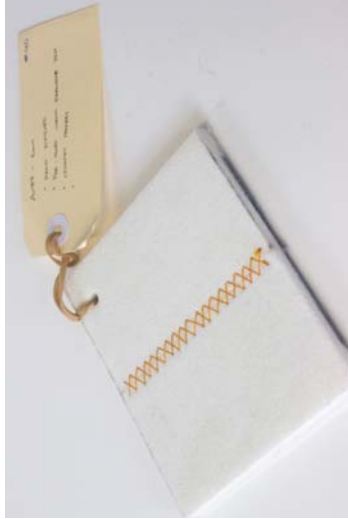
Figure 84 Material: Autex Workstation 6mm / Cotton thread. Test: Stitch joint. Aim: Joining two sheets of Autex with zero waste. Results: A flexible joint was achieved using a cross stitch pattern. Process is zero waste.
