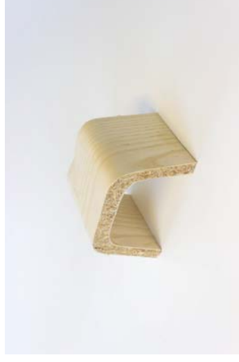
Figure 317 The U shaped mycelium-veneer part after moulding.
