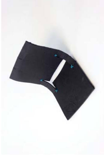
Figure 143 Material: Card / Cotton thread. Test: Stitch detailing as a functional design consideration. Aim: Stop the chair joint from cracking by introducing an aesthetic stitching detail. Results: The criss cross pattern stitched into the stress points on the chair model make an attractive aesthetic detail.
