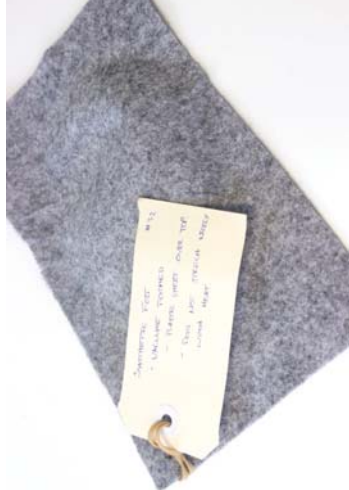
Figure 70 Material: Synthetic felt. Test: Vacuum formed with sacrificial thermoplastic over top. Aim: Adding structure and value to textiles. Results: Felt doesn't stretch very much even with heat. The moulded form didn't add structure to the material. Process is zero waste.
