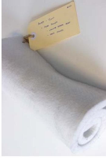
Figure 75 Material: Autex CubeTM 12mm. Test: Heat rolled. Aim: Controlled shaping of the panel product. Results: Autex is pliable when heat is applied. Once the plastic cools down, it forms to the new shape. Process is zero waste.
