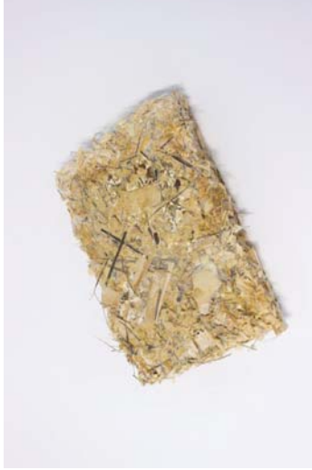
Figure 250 Once removed from the incubator, the sample is ready to be baked to 'kill' the growth of the fungus. While drying, the block can be pressed into a denser board.
