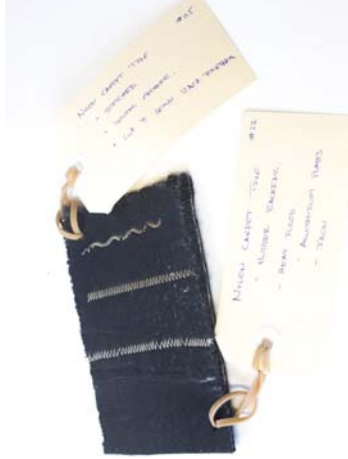
Figure 103 Material: Nylon carpet tile / Cotton thread. Test: Stitch pattern variations using sewing machine. Aim: Experiment with stitching details on carpet. Results: Great material contrast between carpet and thread. Process is zero waste.
