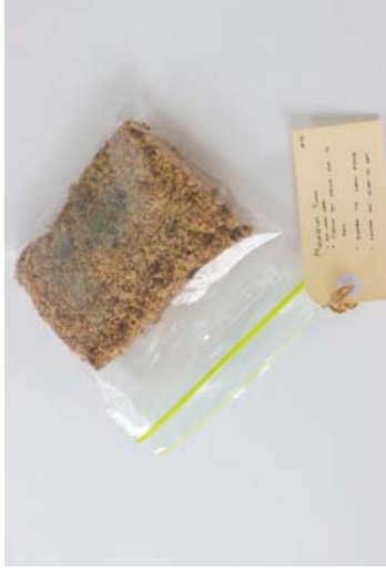
Figure 131 Material: Mycelium / Ash wood waste. Test: Making a lightweight, natural composite material. Aim: Exploring possibilities of growing materials. Results: The new composite material is lightweight. At some point, the sample became contaminated and started to grow bacteria.
