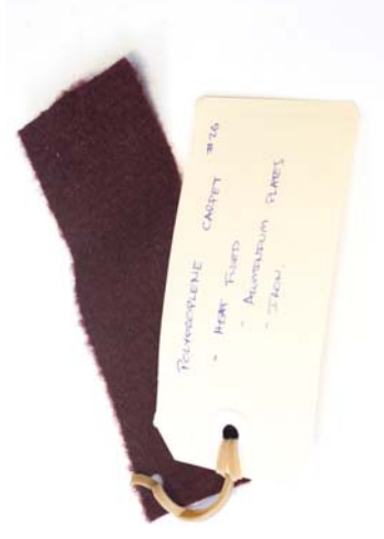
Figure 64 Material: Polyester backless boat carpet. Test: Heat pressed using iron and aluminum plates on one side. Aim: Adding structure and value to carpet waste. Results: Textile rigidity improvement, non-heat pressed side still has grain pattern visible. Process is zero waste.
