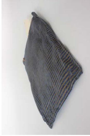
Figure 130 Material: Waste cotton textile / Expanding foam. Test: Making moulded lightweight complex composites. Aim: Exploring possibilities of 3D composites. Results: The new composite material is lightweight and strong. The foam provides some sponginess. The moulding process is zero waste.
