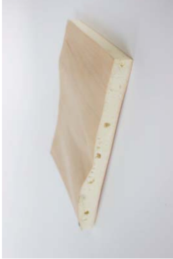
Figure 127 Material: Oak veneer / Expanding foam. Test: Making lightweight, complex-surfaced timber panels. Aim: Exploring possibilities of veneer composites. Results: The new composite material is lightweight and strong. The foam provides some sponginess. The moulding process is zero waste.
