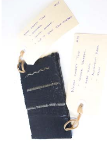
Figure 60 Material: Nylon carpet tile. Test: Heat pressed using iron and aluminum plates. Aim: Adding structure and value to waste carpet tiles. Results: Carpet tiles have a third backing layer that increases the rigidity. Heat pressing the surface increases the strength even more.
