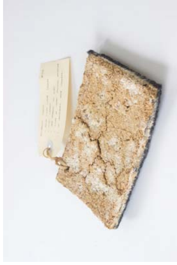
Figure 141 Material: Mycelium / Ash wood waste / Wool carpet. Test: Making a lightweight, grown composite material. Aim: Exploring possibilities of growing materials. Results: The new composite material is lightweight. Once grown with the carpet, the sample was pressed into a dense board.
