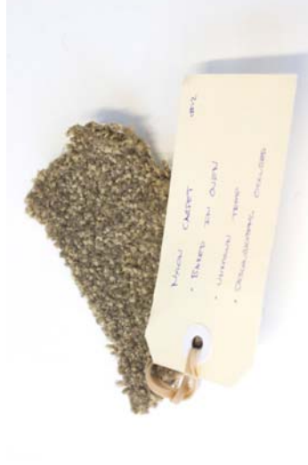
Figure 50 Material: Nylon carpet. Test: Baked in oven. Aim: Melting nylon carpet into forms. Results: Carpet discolored from gray to brown, with slight burnt smell. No fibres melted. Latex bonding agent shrank and became brittle. Process is zero waste.
