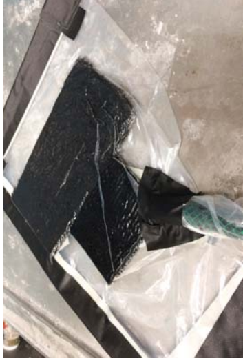
Figure 186 Infusing carpet with epoxy resin in a vacuum bag.
