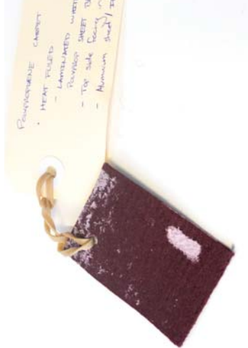
Figure 66 Material: Polyester backless boat carpet / Polypropylene sheet. Test: Heat pressing polypropylene between waste carpet. Aim: Adding structure and value to carpet waste. Results: Textile rigidity increased dramatically. Good bond between textiles. Thin and lightweight composite material. Process is zero waste.
