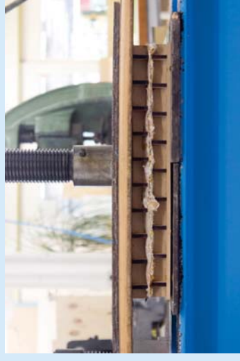
Figure 336 Mycelium-veneer composite in a mould under a hydraulic press.
