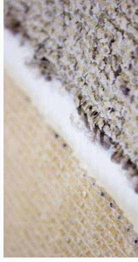
Figure 180 Deconstructed nylon carpet. The secondary backing has been peeled off the back side of the carpet; exposing the latex bonding agent infused into the nylon carpet fibres.
