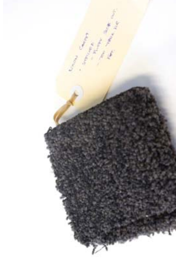
Figure 102 Material: Nylon Carpet / Cotton thread. Test: Stitched two layers of carpet fibre side out. Aim: See what effects can be made using a sewing machine. Results: The two layers of carpet struggled to get underneath the foot of the sewing machine. The carpet fibres engulf the stitching details.
