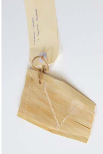
Figure 95 Material: Timber veneer / Cotton thread. Test: Sewing machine stitching patterns. Aim: Alternative material joining technique. Results: Aesthetic joining technique. Process is zero waste.
