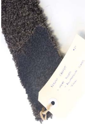
Figure 59 Material: Nylon carpet. Test: Heat pressed using iron and aluminum plates. Aim: An alternative to tinfoil for non-stick heat transfer. Results: Carpet is easily peeled off the aluminum plates. The plates can be re-used. Process is zero waste.
