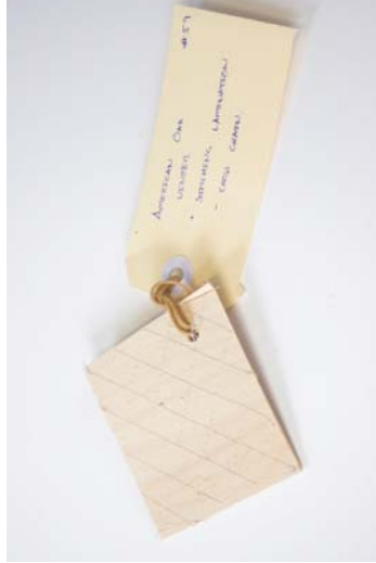
Figure 97 Material: Oak veneer / Cotton thread. Test: Stitched laminate. Aim: Alternative veneer lamination technique. Results: Aesthetic lamination technique. Process is zero waste.
