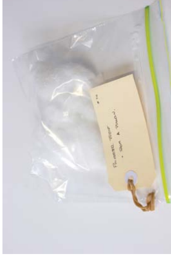
Figure 112 Material: Polyester fibre. Test: Raw material from inside of pillows. Aim: Explore felting capabilities of the fibres. Result: Easily separable and fluffed.
