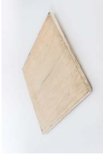
Figure 232 Composite seat base exploration. This sample was overfilled with expanding foam and many of the moulding details didn't come out on the sample.
