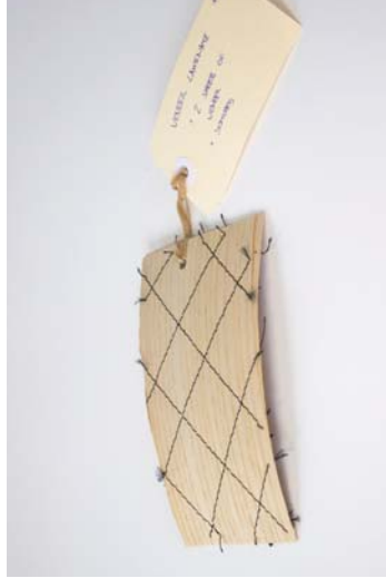
Figure 41 Material: Oak veneer / Cotton thread. Test: Stitched laminate. Aim: Alternative veneer lamination technique. Results: Aesthetic lamination technique. Process is zero waste.
