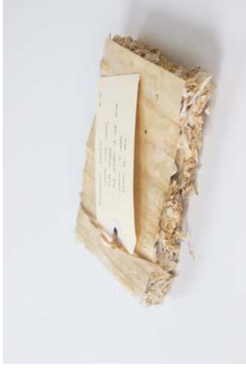
Figure 163 Material: Mycelium / Pine wood waste / Flax fibre / Ash veneer. Test: Making a lightweight, natural composite material. Aim: Adding strength to the mycelium by adding flax fibre. Results: The flax turns out to have anti-fungal properties that limit the growth of mycelium.
