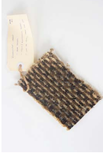
Figure 123 Material: Polypropylene carpet. Test: Heat pressed using iron and aluminum plates. Aim: Adding structure and value to waste carpet. Results: Polypropylene has a much lower melting point than nylon. The original textile pattern is visible in the heat pressed material. Process is zero waste
