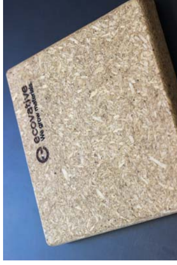
Figure 240 Ecovative MycoBoard. Mycelium and organic matter, pressed into a hard particle board.
