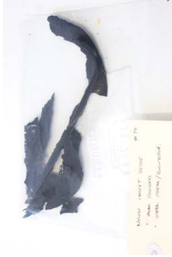
Figure 114 Material: Nylon carpet. Test: Melted carpet fibre. Aim: Creating structure from waste carpet fibre. Results: Heat and pressure is able to melt the loose carpet fibre into rigid plastic forms. The thin sheets are brittle and prone to snapping.
