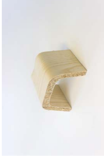
Figure 162 Material: Ecovative mycelium sample / Ash veneer. Test: Mycelium laminate. Aim: Moulding the mycelium laminate into a curved surface. Results: The veneer layer provides great strength improvements while maintaining the materials flexibility. When forced, the mycelium begins to pull away from the veneer.
