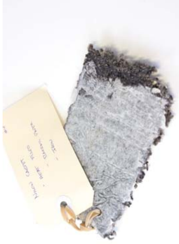
Figure 56 Material: Nylon carpet. Test: Heat pressed using iron and baking paper. Aim: An alternative to tinfoil for non-stick heat transfer. Results: The baking paper was less resistant to fusing with the carpet than tinfoil.
