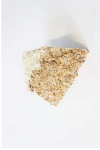
Figure 155 Material: Ecovative mycelium sample. Test: Rip test. Aim: Testing strength properties of mycelium. Results: With some force, a section is able to be ripped from the block.
