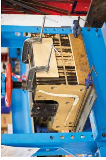
Figure 338 The mycelium and veneer laminate is placed into the mould.
