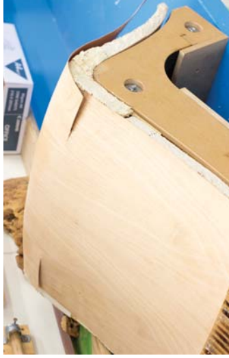
Figure 342 A sheet of veneer placed on the back surface of the chair in preparation for moulding. Two relief cuts are required for the veneer to form around the compound surface.
