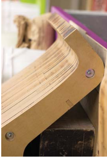
Figure 320 Sanding back the stepped layers to a smooth mould surface.
