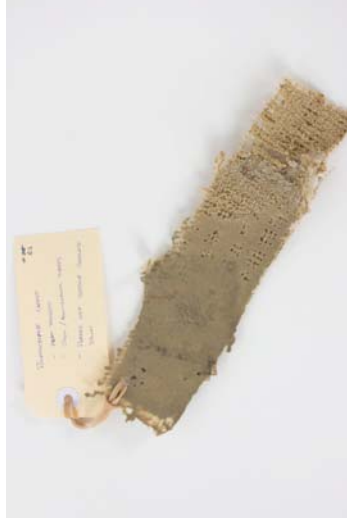
Figure 121 Material: Polypropylene carpet. Test: Heat pressed using iron and aluminum plates. Aim: Adding structure and value to waste carpet. Results: Polypropylene has a much lower melting point than nylon. The fibres melt down into a smooth surface. Process is zero waste.
