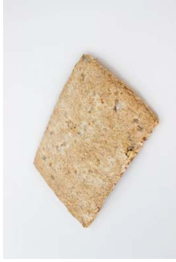
Figure 133 Material: Mycelium / Ash wood waste. Test: Making a lightweight, natural composite material. Aim: Exploring possibilities of growing materials. Results: The new composite material is lightweight. Once grown, the sample was pressed into a dense board.
