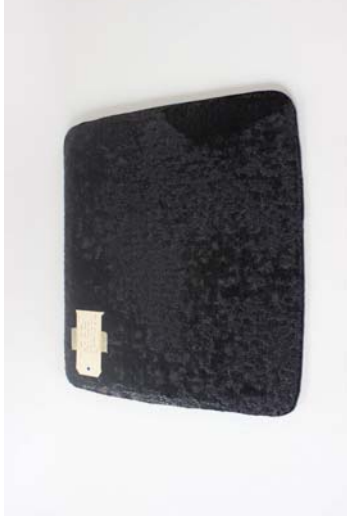
Figure 148 Material: Nylon carpet / Epoxy resin. Test: Intusing carpet with epoxy resin to craft a seat base. Aim: Adding structure and value to waste carpet. Results: The new composite material is lightweight and strong, but too flexible for a seat base.
