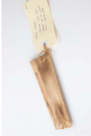
Figure 137 Material: Oak veneer. Test: Heat forming timber veneer with iron. Aim: To make veneer more malleable for moulding. Results: The iron discoloured the veneer. It flattened the bumps in ripples in the surface, but was not able to be flexed into shape post heating.
