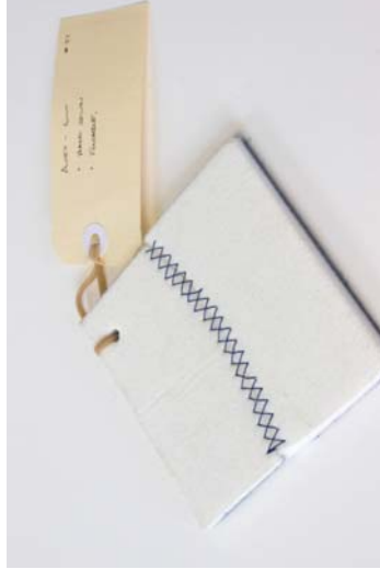
Figure 89 Material: Autex Workstation 6mm / Cotton thread. Test: Stitch joint around radius. Aim: Joining two sheets of Autex with zero waste. Results: A flexible joint was achieved using a cross stitch pattern. Process is zero waste.
