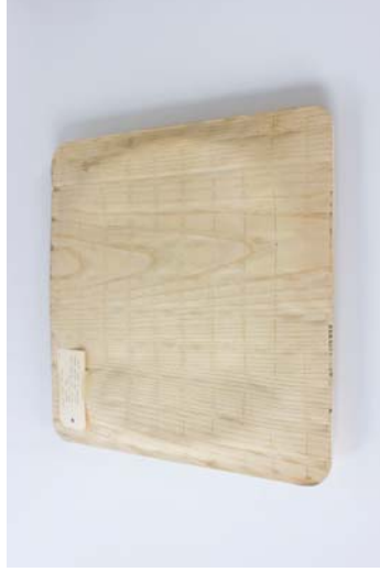
Figure 150 Material: Oak veneer / Poplar ply / Expanding foam. Test: Veneer foam seat base #2. Aim: Craft a compound-surfaced seat base, using the veneer / expanding foam method, that is strong enough to support a person. Results: After learning from the last attempt, this one moulded far better. The quilted effect came from the lattice mould.
