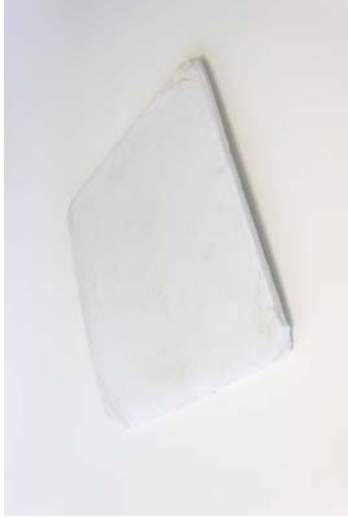
Figure 195 An Autex Cube™ seat base moulded using the MDF mould used in the carpet composite concept. Even though the sheet has been formed into a compound surface, the panel is not rigid enough to support a person.
