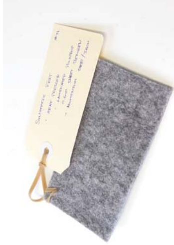
Figure 69 Material: Synthetic felt / Polypropylene sheet. Test: Heat pressed using iron and aluminum plates. Aim: Adding structure and value to textiles. Results: Felt doesn't fuse with the polypropylene very well. Easily delaminated. Process is zero waste.
