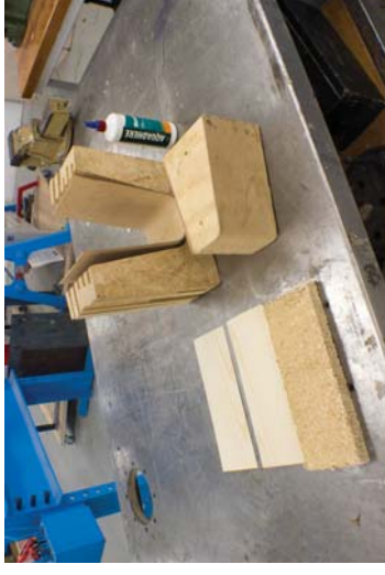
Figure 315 The test mould components laid out ready to press.
