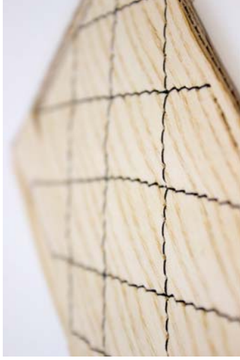
Figure 226 Quilted timber veneer with a corrugated cardboard substrate.
