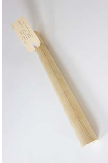
Figure 145 Material: Ash veneer / poplar ply / expanding foam. Test: Chair leg. Aim: Craft a chair leg, using the veneer / expanding foam method that it strong enough to support a person. Results: Due to overfilling the cavity with too much foam, the veneer split at the seam, making the tapered cylinder non-uniform.
