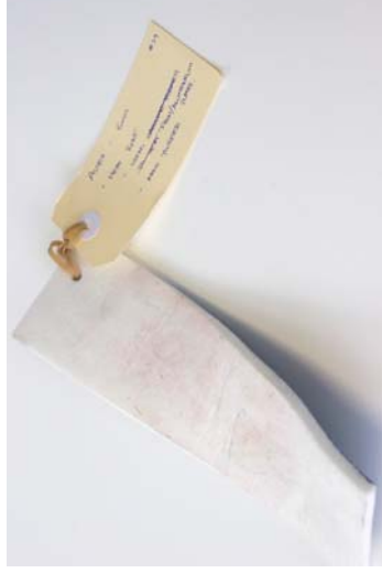
Figure 77 Material: Autex Workstation 6mm. Test: Boiling water forming. Aim: Controlled shaping of the panel product. Results: Autex is pliable when its exposed to boiling water. The material must be held in a form until it dries. Process is zero waste.
