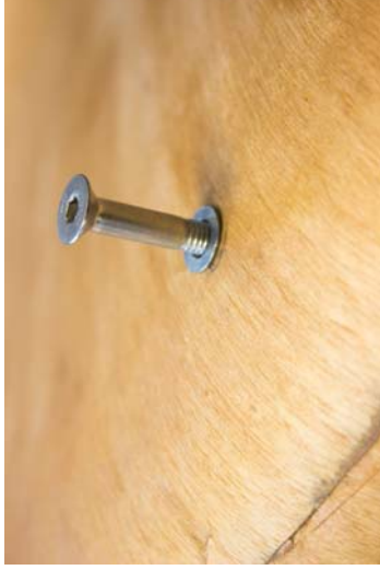
Figure 348 Insert nuts threaded into the void provide a strong anchor to fasten the seat base to the legs.
