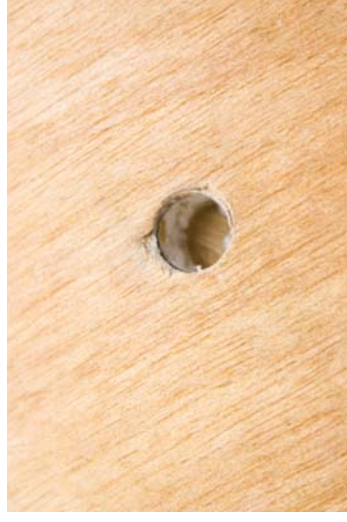
Figure 347 The veneer circle is visible indented into the mycellium substrate.
