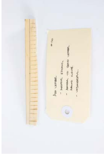
Figure 168 Material: Ash Veneer. Test: Zero waste kerfing. Aim: Bend veneer around curved surfaces without creating waste. Results: The veneer is still much too brittle to flex around a bend without snapping.
