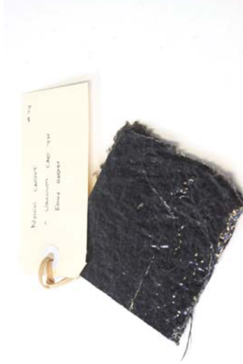
Figure 116 Material: Nylon carpet / Epoxy resin. Test: Infusing carpet with epoxy resin. Aim: Adding structure and value to waste carpet. Results: The new composite material is lightweight and strong. The surface is glossy, much like ripples on water.
