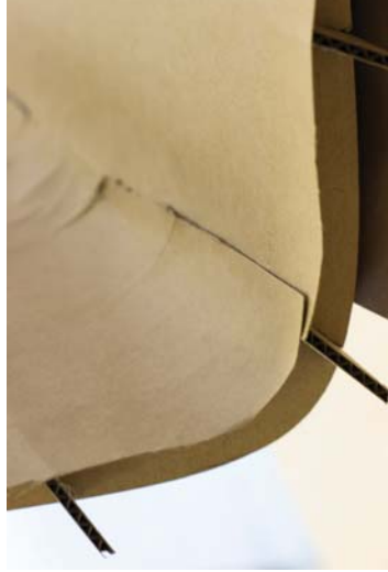
Figure 310 Relief cut on the Peel/Pare cardboard model.
