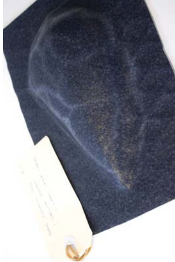
Figure 73 Material: Linooleum flooring tile. Test: Vacuum formed. Aim: Adding structure and value to wasted flooring materials. Results: Lino flooring tiles are made from multiple layers of varying materials. Some melt quicker than others. A latex component cracks under the surface. Process is zero waste.
