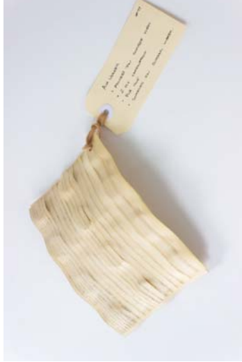
Figure 135 Material: Ash veneer. Test: Compound surface moulding. Aim: To mould compound curves into timber veneer. Results: Compound surfaces are plausible in timber veneer. The grain allows the surface to expand and contract to get around the ridges in the mould. Veneer is prone to splitting along the grain.
