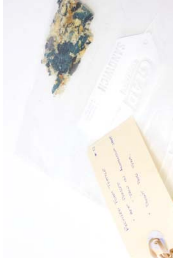
Figure 90 Material: Recycled foam moving blanket. Test: Heat pressed using iron and aluminum plates. Aim: Adding structure and value to textile waste. Results: Foam did not react to the heat and pressure. No change in material properties. Process is zero waste.
