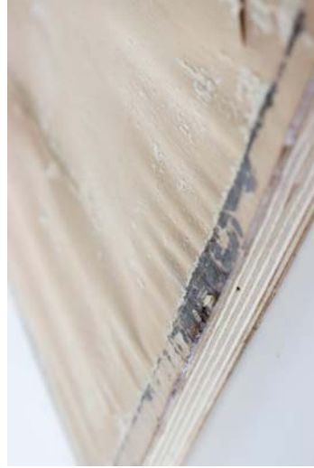
Figure 233 The laminate was glued down around the edges of the panel. When it was filled with foam, some interesting stretch patterns were formed.
