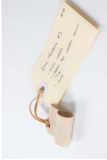
Figure 136 Material: Oak veneer. Test: Radius edge finishing with 2-ply of veneer. Aim: To experiment with finishing the veneer edges. Results: Two layers of veneer were wrapped and glued around a steel rod. The veneer is very flexible when curved in one direction in line with the grain.
