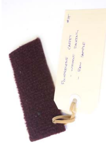
Figure 63 Material: Polyester backless boat carpet. Test: Raw sample. Aim: Experiment with adding structure and value to carpet that has no other infused materials such as latex.
