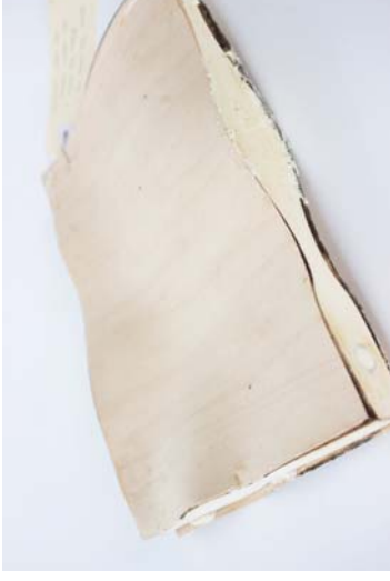
Figure 229 Expanding foam veneer composite with an external frame. The frame increases the strength of the form without adding much more mass.
