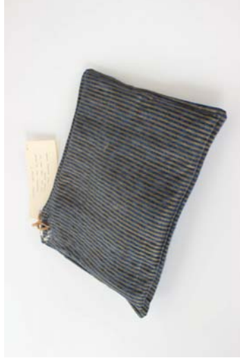
Figure 129 Material: Waste cotton textile / Expanding foam. Test: Making lightweight complex composites. Aim: Exploring possibilities of 3D composites. Results: The new composite material is lightweight and strong. The foam provides some sponginess. The moulding process is zero waste.
