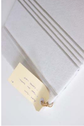
Figure 39 Material: Autex Cube™ 12mm. Test: Saw kerfing. Aim: Controlled shaping. Results: Makes the semi-rigid panel bendable in one direction. The process creates waste in the removal of material.
