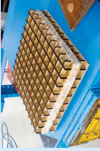
Figure 335 Mycelium-veneer composite sample ready for pressing.
