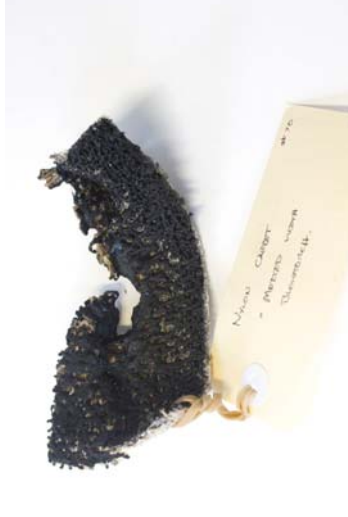
Figure 108 Material: Nylon carpet. Test: Melting carpet using a blowtorch. Aim: Melt the nylon fibres into a block for further use. Results: The carpet composite shrivelled and burned. The melted textile has no further application.
