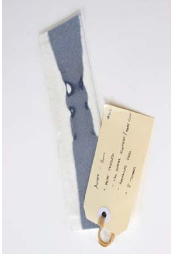
Figure 80 Material: Autex Workstation 6mm. Test: Heat pressing. Aim: Controlled shaping of the panel product. Results: A press squashed the 6mm panel down to 3mm, improving its rigidity. Process is zero waste.
