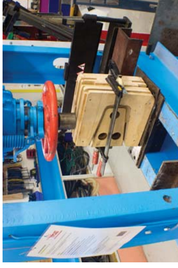
Figure 316 Moulding the composite into a U shape that represents the legs of the chair.
