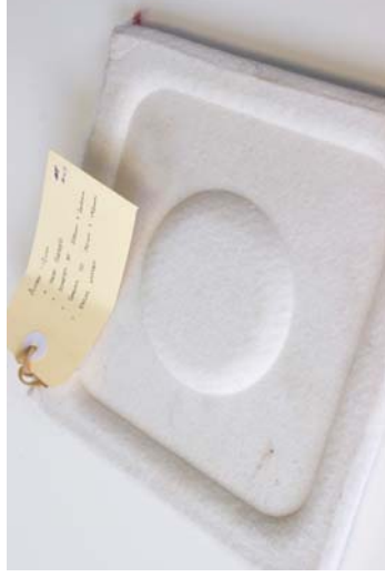
Figure 85 Material: Autex Cube™ 12mm. Test: Heat pressing. Aim: Controlled shaping of the panel product. Results: Crisp details exposed in moulding. The panel shrank slightly when heated. Process is zero waste.
