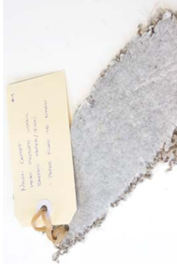
Figure 57 Material: Nylon carpet. Test: Heat pressed using iron and baking paper. Aim: An alternative to tinfoil for non-stick heat transfer. Results: The baking paper was less resistant to fusing with the carpet than tinfoil.
