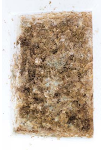
Figure 174 Material: Mycelium / Coffee husks. Test: Making a lightweight, natural composite material. Aim: Exploring possibilities of growing materials. Results: The new composite material is lightweight, yet very brittle.
