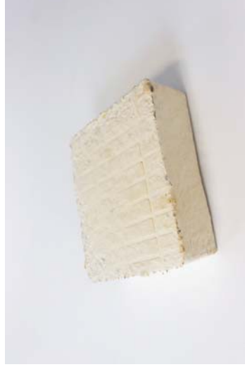
Figure 238 Ecovative mycelium block. Measures approximately 150mm x 160mm x 50mm.
