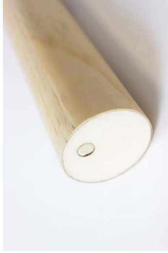
Figure 146 Material: Ash veneer / Poplar ply / Expanding foam. Test: Chair leg #2. Aim: Craft a chair leg, using the veneer / expanding foam method, that is strong enough to support a person. Results: This one turned out much better. The veneer nicely butts up the whole length of the leg.
