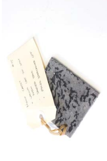
Figure 117 Material: Nylon carpet / Epoxy resin. Test: Sanding back epoxy carpet composite. Aim: Changing the surface texture of waste carpet composite. Results: The new composite material is lightweight and strong. The surface is glossy, much like ripples on water.
