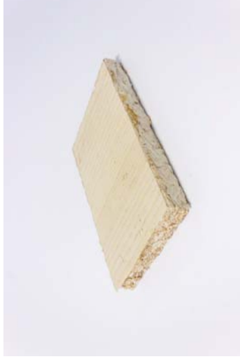
Figure 156 Material: Ecovative mycelium sample / Ash veneer. Test: Mycelium laminate. Aim: Increasing strength properties of mycelium. Results: The veneer layer provides great strength improvements while maintaining the materials flexibility.
