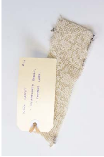
Figure 52 Material: Nylon carpet. Test: Carpet deconstruction. Aim: Exposing alternative functions of carpet. Results: Interesting pixelated aesthetics are exposed where the latex bonding agent is left joined to the backing. Process is zero waste.
