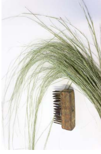
Figure 247 A heckling comb is used to separate the flax fibres into individual strands. The process is slow by hand, but industrial flax mills process flax quickly and efficiently.
