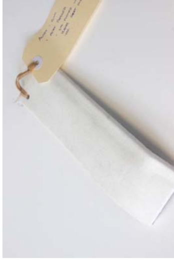
Figure 76 Material: Autex Workstation 6mm. Test: Vacuum formed with sacrificial plastic sheet on top. Aim: Adding structure and value to wasted flooring materials. Results: The Autex formed to the shape, but the details in the moulding don't show up very much. Process is zero waste.
