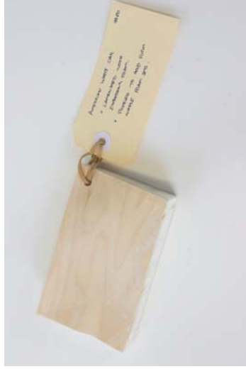
Figure 118 Material: Oak veneer / Expanding foam. Test: Making lightweight, complex-surfaced timber panels. Aim: Exploring possibilities of veneer composites. Results: The new composite material is lightweight and strong. The foam provides some sponginess. The moulding process is zero waste.
