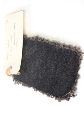
Figure 58 Material: Nylon carpet. Test: Heat pressed using iron and aluminum plates. Aim: An alternative to tinfoil for non-stick heat transfer. Results: Carpet is easily peeled off the aluminum plates. The plates can be re-used. Process is zero waste.
