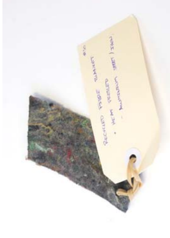
Figure 68 Material: Recycled textile blanket. Test: Heat pressed using iron and aluminum plates. Aim: Adding structure and value to textile waste. Results: Textile rigidity improvement; due to the mixture of textile composition, some fibres melt and others do not. Process is zero waste.
