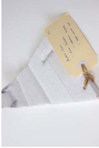
Figure 40 Material: Autex Cube™ 12mm. Test: Pressed fold. Aim: Controlled shaping. Results: Presses a recess into the surface. The panel product is bendable on the pressed areas. Shorter pressed areas can be aesthetic details. Process is zero waste.
