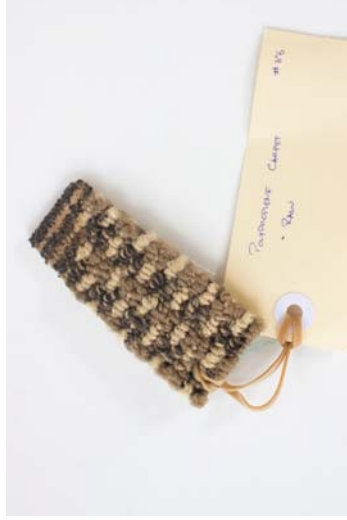
Figure 122 Material: Polypropylene carpet. Test: Raw carpet. Aim: Compare heat pressed pattern to original textile.
