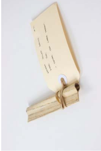
Figure 159 Material: Ash veneer. Test: Rolling test. Aim: Experiment with the flexibility limits of veneer. Results: Veneer set and rolled around a steel rod to dry. The faces were glued together to maintain its shape.
