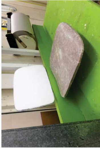
Figure 219 Form study prototyping for the rotationally moulded Pillow Chair using polystyrene foam and paper maché.
