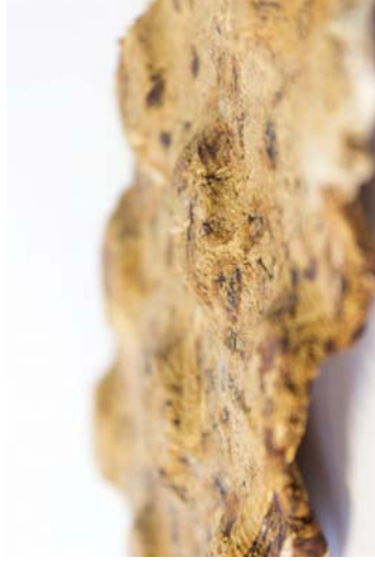
Figure 255 Mycelium and natural wood fibres, press moulded into a complex surface.
