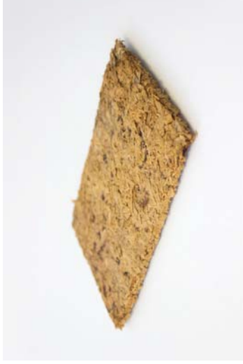
Figure 244 Heat pressed: a block of mycelium and Ash wood shavings. The 100% natural fibre board has an almost edible quality about it.
