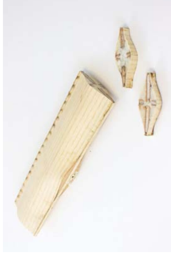
Figure 269 Sample section of expanding foam consuming the cardboard skeleton within the veneer skin.
