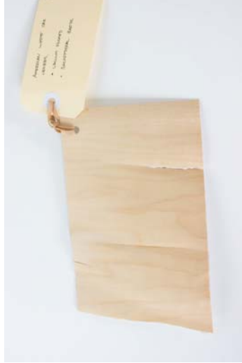
Figure 126 Material: Oak veneer. Test: Vacuum formed with sacrificial thermo-plastic layer. Aim: Creating complex surfaces in timber veneer. Results: The veneer was not able to flex into complex surfaces without fracturing.
