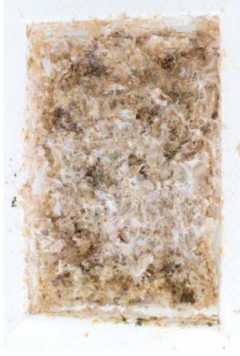
Figure 251 Mycelium grown in coffee husks.
