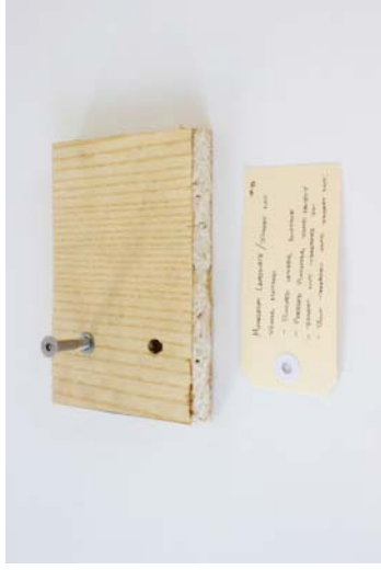
Figure 171 Material: Mycelium / Ash veneer / Insert nut. Test: Zero waste fixings. Aim: Provide a strong fixing method that created zero waste. Results: A circle is pressed into the mycelium surface, creating a cavity into which an insert nut can be threaded. The nut provides a strong anchor point for attaching the components to each other.
