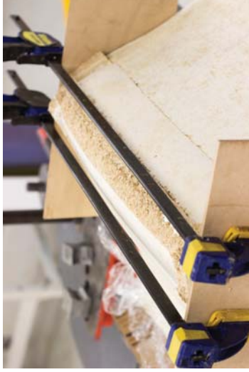
Figure 341 The fractured section was cut out and replaced with two straight pieces with a butt joint. Custom grown mycelium would resolve this issue.
