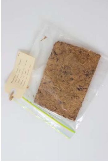
Figure 132 Material: Mycelium / Ash wood waste. Test: Making a lightweight, natural composite material. Aim: Exploring possibilities of growing materials. Results: The new composite material is lightweight. Once grown, the sample was pressed into a dense board.
