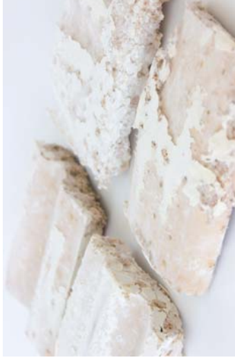
Figure 253 Mycelium grew in wood waste, faced with timber veneer. These samples are grown for 5 weeks within a dark and humid environment. During the growing process, the mycelium passes through the veneer and starts to grow on the external surfaces.
