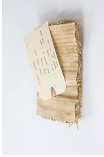
Figure 165 Material: Mycelium / Pine wood waste / Flax fibre / Ash veneer. Test: Making a lightweight, natural composite material. Aim: Adding strength to the mycelium by adding flax fibre. Results: Pressing the mycelium improved its strength, but still not as strong as previous tests.
