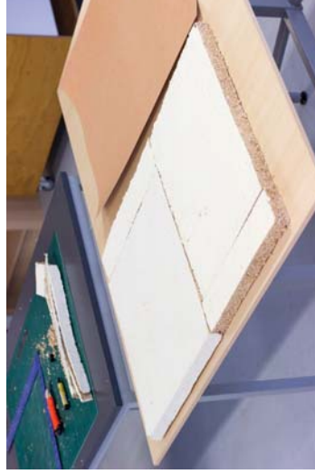
Figure 327 Laying out the mycelium substrate into the sheet size in preparation for lamination. In production, custom grown mycelium panels would be grown to size.
