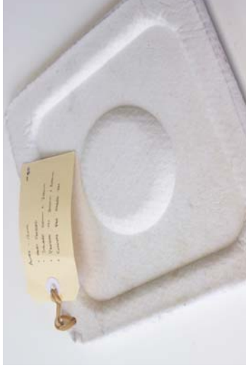
Figure 88 Material: Autex Cube™ 12mm. Test: Heat pressing. Aim: Controlled shaping of the panel product. Results: Crisp details exposed in moulding. The oversize panel shrank slightly when heated to fit the cavity. Edges were pushed into form the radius. Process is zero waste.
