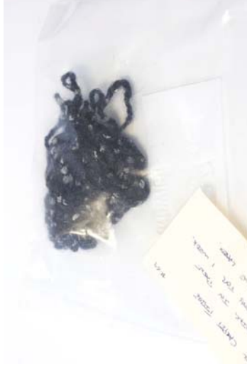
Figure 107 Material: Wool carpet. Test: Carpet deconstruction. Aim: Dissolving the latex off the wool fibres. Results: Soaking the wool in acetone for three weeks softened the latex, but did not dissolve it off all together.
