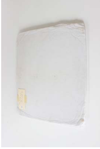
Figure 147 Material: Autex Cube™ 12mm. Test: Heat pressed seat base. Aim: Controlled shaping of the panel product. Results: Heated up under element, then transferred into the press mould. The panel took the shape of the compound surfaced mould with ease.
