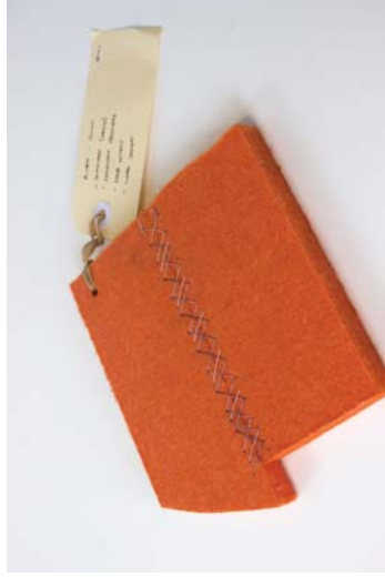
Figure 62 Material: Autex Cube™ 12mm / Cotton thread. Test: Stitch joint. Aim: Joining two sheets of Autex with zero waste. Results: A flexible joint was achieved using a cross stitch pattern. Process is zero waste.
