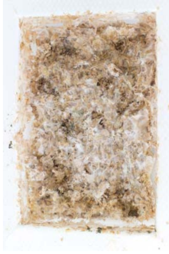
Figure 173 Material: Mycelium / Coffee husks. Test: Making a lightweight, natural composite material. Aim: Exploring possibilities of growing materials. Results: The new composite material is lightweight, yet very brittle.
