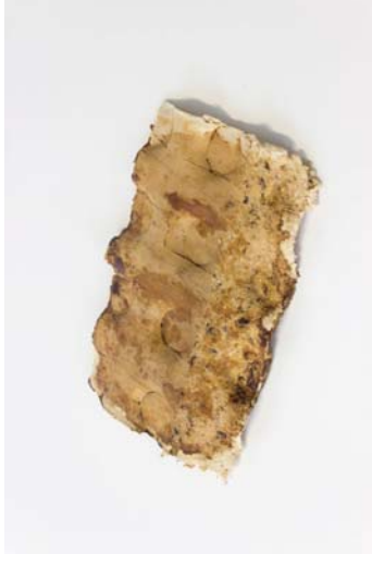
Figure 254 One of the mycelium samples heat pressed in a two-part mould. The sample becomes much more rigid with the added veneer and compound surface.
