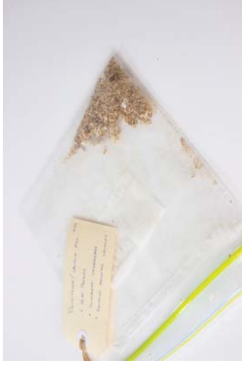
Figure 92 Material: Wood and polystyrene waste from fabrication workshop. Test: Heat pressed using iron and aluminum plates. Aim: Experiment with adding structure and value to a mixture of wasted particles. Results: Polystyrene beads shrank and infused the wood waste. Resultant composite material is crumbly
