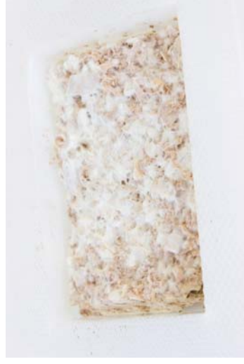
Figure 243 Mycelium after roughly 3 weeks of growth in waste Ash wood shavings.
