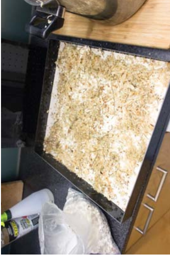
Figure 256 Mixing waste wood chips, flax fibre and mycelium to grow in between timber veneer. It is important to maintain a sterilised environment to reduce contamination while preparing the material's growth.
