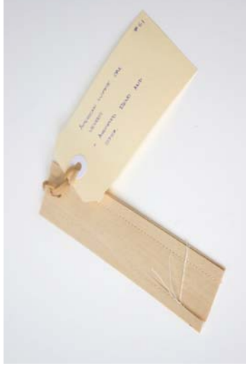
Figure 98 Material: Timber veneer / Cotton thread. Test: Stitched together two veneer sheets while bent. Aim: Stitch veneer into a complex form. Results: Due to the size of the sample, the sheets don't stay curved when sewn. Process is zero waste.
