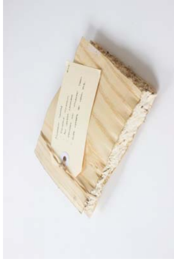
Figure 157 Material: Ecovative mycelium sample / Ash veneer. Test: Mycelium compound-surfaced laminate. Aim: Increasing strength properties of mycelium. Results: The veneer layer provides great strength improvements while maintaining the material's flexibility. The 3D mould imparted the lattice structure into the veneer.
