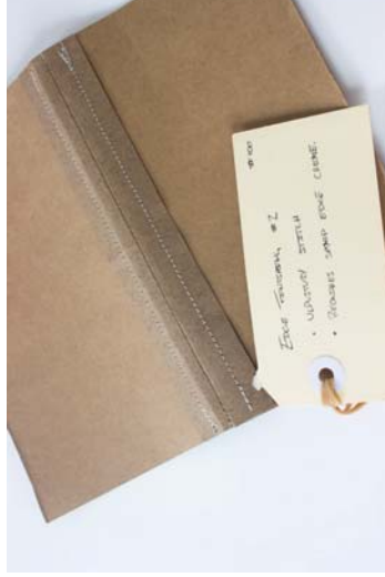
Figure 138 Material: Kraft paper / Cotton thread. Test: Upholstery stitch. Aim: Exploring possibilities of joining and finishing material edges. Results: Contrasting material textures and colours. Strong joint that hides the unclean edge. Process is zero waste.
