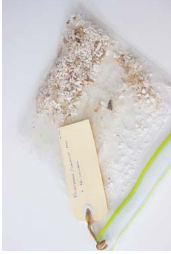
Figure 91 Material: Wood and polystyrene waste from fabrication workshop. Test: Raw sample. Aim: Experiment with creating composite materials from waste materials. Result: The materials are well mixed.
