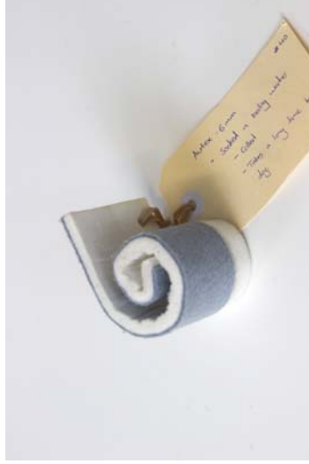
Figure 78 Material: Autex Workstation 6mm. Test: Boiling water forming. Aim: Controlled shaping of the panel product. Results: Autex is pliable when its exposed to boiling water. The material must be held in a form until it dries. Process is zero waste.
