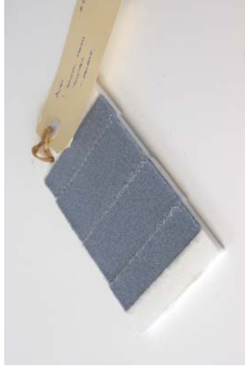
Figure 98 Material: Autex Workstation 6mm / Cotton thread. Test: Stitch joint variations using sewing machine. Aim: Joining two sheets of Autex with zero waste. Results: A flexible joint was achieved using a cross stitch pattern. Process is zero waste.
