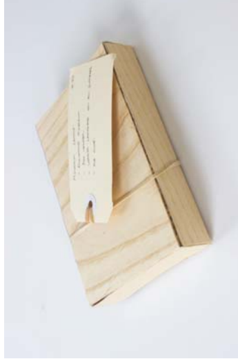
Figure 161 Material: Ecovative mycelium sample / Ash veneer. Test: Mycelium laminate. Aim: Increasing strength properties of mycelium. Results: The veneer layer on all sides provides great strength improvements. It's difficult to maintain uniform edges.
