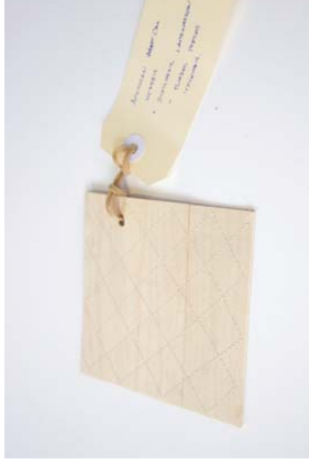
Figure 96 Material: Oak veneer / Cotton thread. Test: Stitched laminate. Aim: Alternative veneer lamination technique. Results: Aesthetic lamination technique. Process is zero waste.
