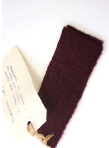
Figure 65 Material: Polyester backless boat carpet. Test: Heat pressing two pieces together. Aim: Adding structure and value to carpet waste. Results: Textile rigidity improvement. Inner surfaces don't bond together very well, easily pulled apart. Process is zero waste.
