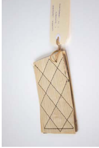
Figure 42 Material: Oak veneer / Cotton thread / Corrugated cardboard. Test: Stitched laminate with substrate. Aim: Added cushion to laminate. Results: Aesthetic lamination technique, with quilted properties. Process is zero waste.
