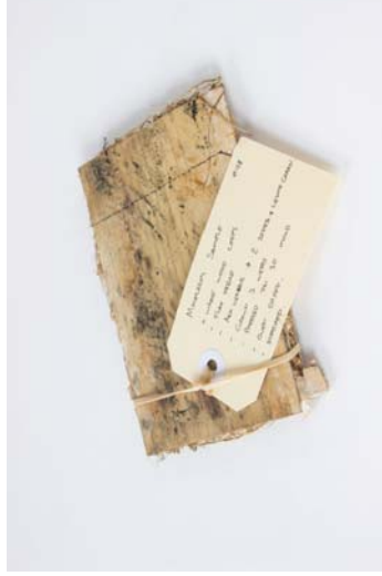
Figure 166 Material: Mycelium / Pine wood waste / Flax fibre / Ash veneer. Test: Making a lightweight, natural composite material. Aim: Adding strength to the mycelium by adding flax fibre. Results: Pressing the mycelium improved its strength, but still not as strong as previous tests.
