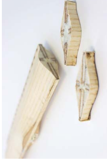
Figure 158 Material: Ash veneer / Corrugated cardboard / Expanding foam. Test: Chair frame. Aim: Craft an organic-surfaced chair frame. Results: A strong structure is obtained when the veneer is moulded in complex surfaces. I cut the sample section to see how the foam filled the cavity.
