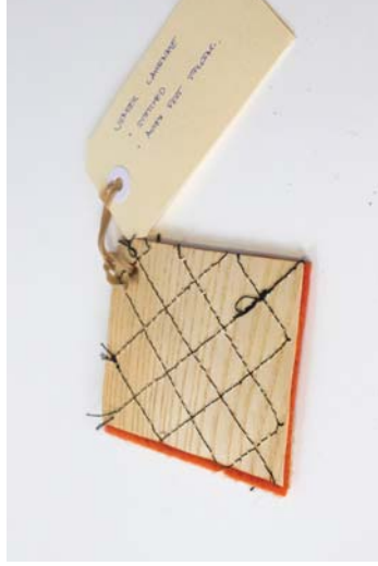
Figure 46 Material: Oak veneer / Cotton thread / Autex Composition®. Test: Stitched laminate with substrate. Aim: Added cushion to laminate. Results: Aesthetic lamination technique. Process is zero waste, but is not recyclable or decomposable as a composite.
