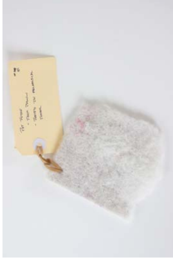
Figure 119 Material: Polyester fibre. Test: Felted in industrial felting machine. Aim: Add structure and rigidity to polyester fibre. Results: Felting polyester fibre meshes the fibres together. Its textile structure increases. Process is zero waste.
