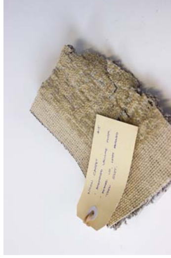
Figure 53 Material: Nylon carpet. Test: Adding structure to carpet waste. Aim: Vacuum form carpet. Results: The latex in the carpet shrinks under heat. The backing starts to become brittle and disintegrates.
