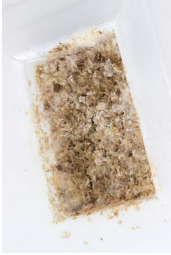
Figure 172 Material: Mycelium / Coffee husks. Test: Making a lightweight, natural composite material. Aim: Exploring possibilities of growing materials. Results: The new composite material is lightweight, yet very brittle.
