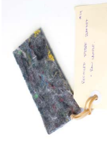
Figure 67 Material: Recycled textile blanket. Test: Raw sample. Aim: Experiment with adding structure and value to waste textiles.
