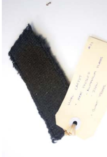
Figure 61 Material: Wool carpet. Test: Heat Pressed using iron and aluminum plates. Aim: See what happens to wool when heat pressed. Results: The wool carpet did not melt like the synthetic carpets. The fibres did press down. Process is zero waste.
