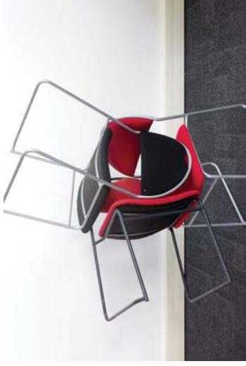
Figure 212 Mocking up how three chair bases and backs can be rotationally moulded as one piece, then cut apart to form three identical chairs.
