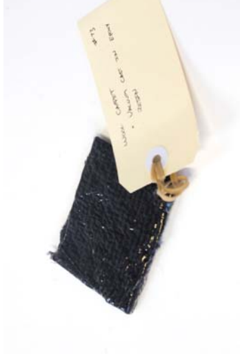
Figure 115 Material: Wool carpet / Epoxy resin. Test: Infusing carpet with epoxy resin. Aim: Adding structure and value to waste carpet. Results: The new composite material is lightweight and strong. The surface is glossy, much like ripples on water. The carpets grain is now much more obvious.
