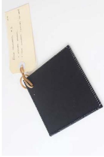
Figure 134 Material: Black card / Cotton thread. Test: Experimenting with edge detailing using thread. Aim: Exploring possibilities of joining and finishing material edges. Results: Contrasting material textures and colours. Process is zero waste.
