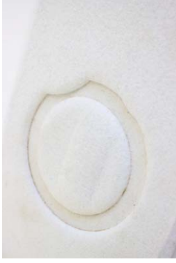
Figure 193 Heat pressed Autex sample. Autex heated in an oven until soft and pliable. An MDF shape was placed on top and pressed in a hydraulic press. The pressed shape is much firmer and more rigid than an unpressed panel.
