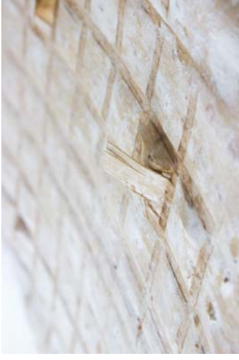
Figure 259 Fractures in the surface veneer occur in areas of narrower panel thickness, where the panel is compressed in an area with large wood chips. The large chips — not able to compress, puncture the veneer surface.
