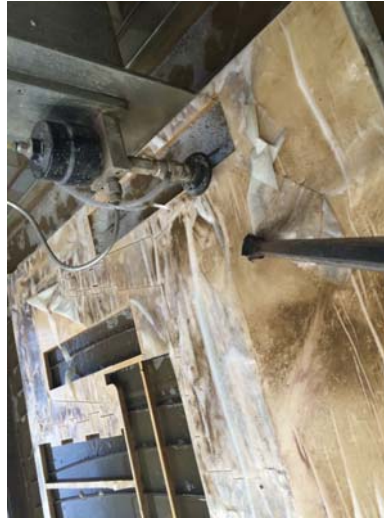
Figure 20 The Strip Chair (2013) is fabricated using a CNC water jet cutter. A layer of adhesive paper was applied to the surface to reduce damage to the surface veneer.
