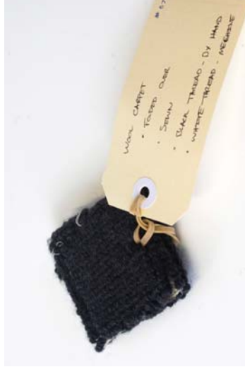
Figure 105 Material: Wool carpet / Cotton thread. Test: Stitched two layers of carpet fibre side out. Aim: See what effects can be made using a sewing machine. Results: The two layers of carpet struggled to get underneath the foot of the sewing machine. The carpet fibres engulf the stitching details.
