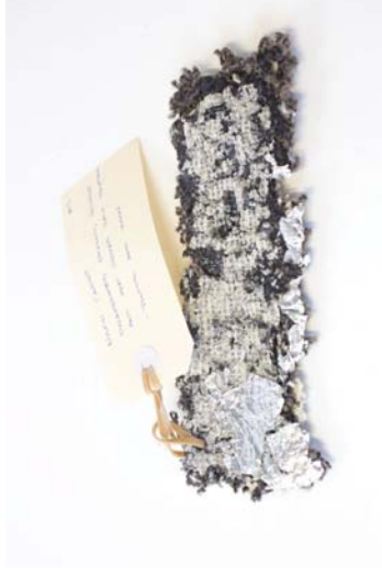
Figure 51 Material: Nylon carpet. Test: Deconstructed and heat pressed using iron and tinfoil. Aim: Adding structure and value to carpet waste. Results: Nylon not fully melted through. Tinfoil fuses to the melted carpet and is difficult to pull off. Ugly backing aesthetic visible. Process is zero waste.
