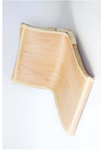
Figure 343 Both the front and back surface veneers are laminated onto the mycelium substrate.
