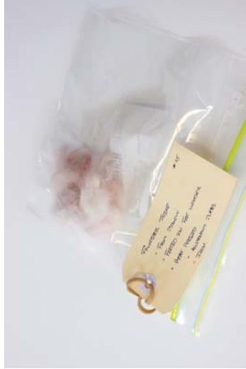
Figure 113 Material: Polyester fibre. Test: Carded and heat pressed. Aim: Add structure and rigidity to polyester fibre. Results: Carding polyester fibre aligns the fibres in a single direction. Difficult to make a rigid structure when heat pressing the mat.
