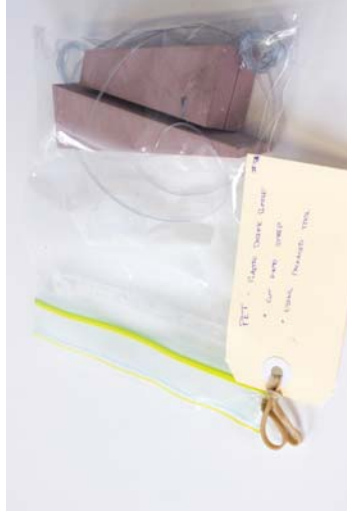
Figure 93 Material: PET plastic bottles. Test: Cut fine threads of plastic. Aim: Cut threads into as fine threads as possible. Results: Using the cutting technique, threads of a minimum of 1mm were capable of being cut.
