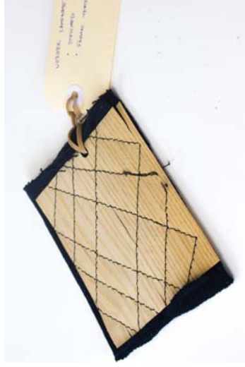
Figure 45 Material: Oak veneer / Cotton thread / Polyester textile. Test: Stitched laminate with substrate. Aim: Added cushion to laminate. Results: Aesthetic lamination technique. Process is zero waste, but is not recyclable or decomposable as a composite.
