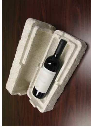
Figure 237 Mycelium packaging. Developed as an alternative to polystyrene foam.
