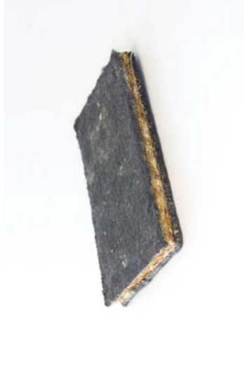
Figure 245 Mycelium with ash wood waste, grown between two layers of wood carpet. The block was heat pressed post growth into a dense fibreboard composite.
