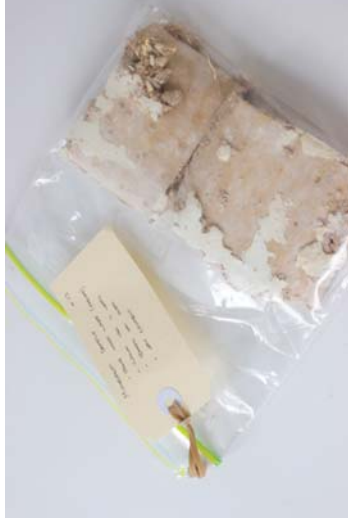
Figure 151 Material: Mycelium / Pine wood waste / Oak veneer. Test: Making a lightweight natural composite material. Aim: Exploring possibilities of growing material laminates. Results: The new composite material is lightweight. Baked in oven to kill growth, sample is very crumbly.
