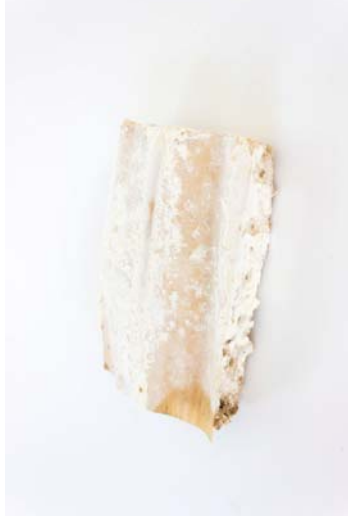
Figure 152 Material: Mycelium / Pine wood waste / Oak veneer. Test: Making a lightweight natural composite material. Aim: Exploring possibilities of growing material laminates. Results: The new composite material is lightweight and strong. The veneer curled up from the moisture of the mycelium growing conditions.
