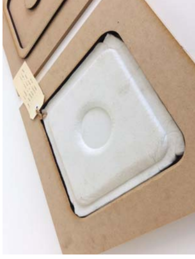
Figure 194 An attempted zero waste moulding of a three-dimensional panel form. Through iterative tests, I explored different methods of moulding a square of Autex into a panel with rounded corners without removing any material.
