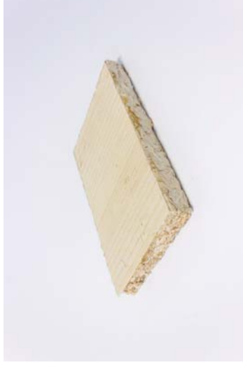
Figure 313 Ecovative mycelium and veneer composite.
