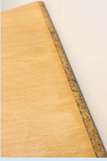
Figure 332 Mycelium substrate extruding beneath veneer.
