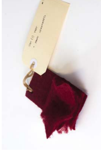
Figure 110 Material: Polyester felt. Test: Deconstructing felt layers. Aim: Separate polyester fibres. Results: The felt separates into layers. The felt easily pulls apart into it fibres.
