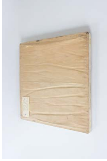
Figure 149 Material: Oak veneer / Plywood / Expanding foam. Test: Veneer / foam seat base. Aim: Craft a compound-surfaced seat base, using the veneer / expanding foam method, that is strong enough to support a person. Results: The veneer stretched and warped along its grain in the mould. This may be due to steaming the timber beforehand.
