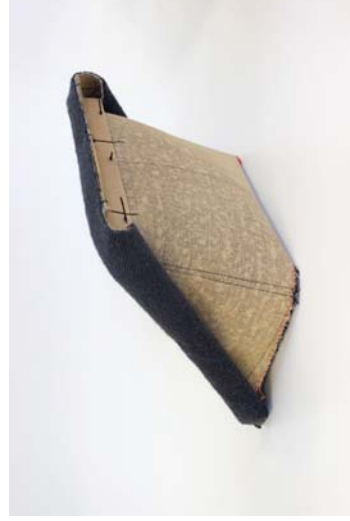
Figure 184 Wool carpet formed into a shell chair structure using rolling and stitching techniques. Bracing was required to support the extra stresses of a human.
