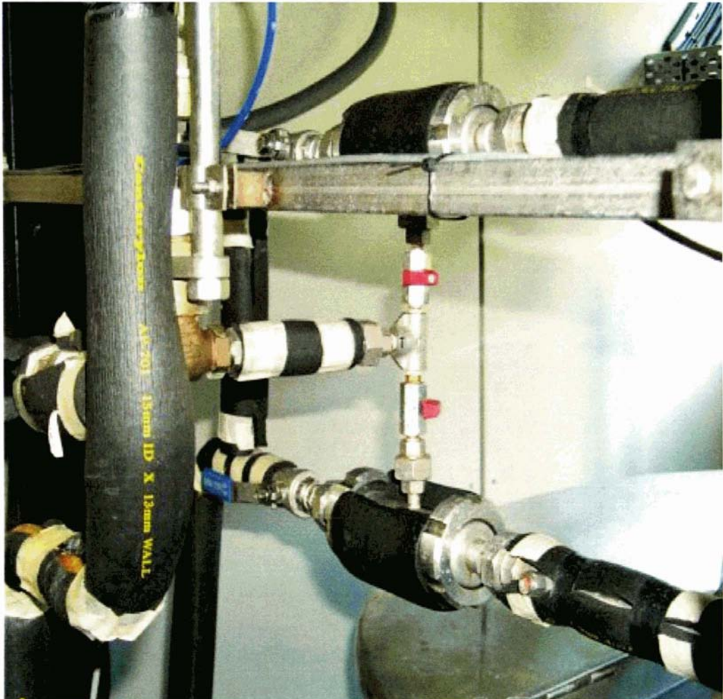
Figure 3.1.3. Photograph showing two of the DSI units installed in the pilot plant.
