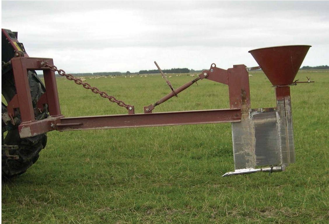
Plate 5.1 Modified mole plough, with the added hopper and delivery chute, used to install tephra into mole channels.
