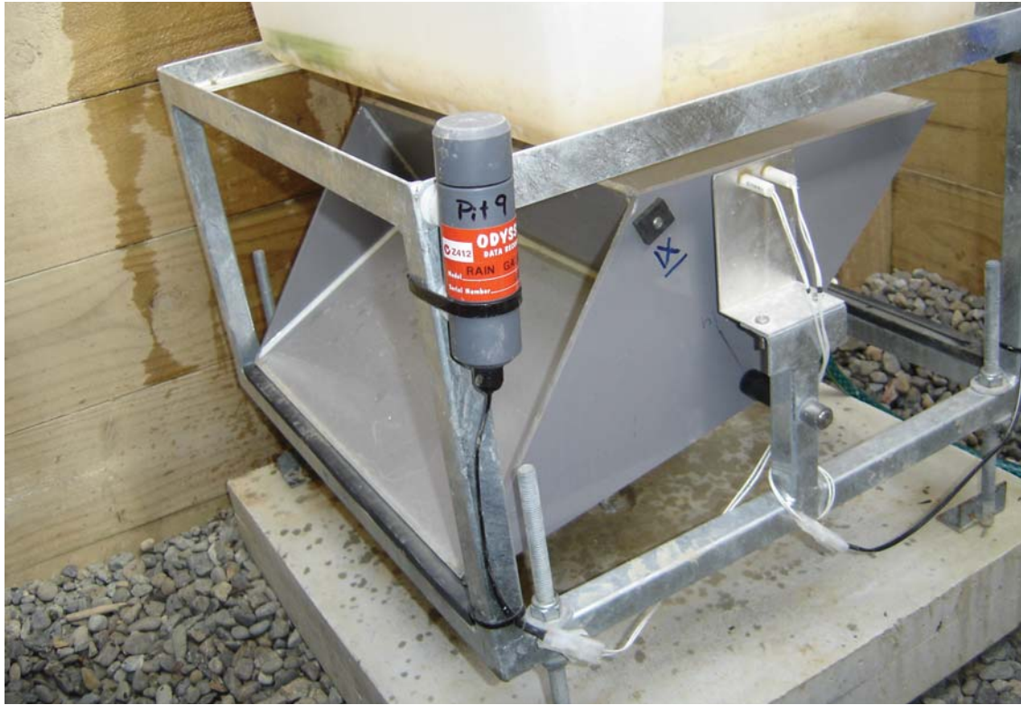
Plate 3.1 An example of a tipping bucket flow meter and data logger used for measuring and recording drainage water flow rates.
