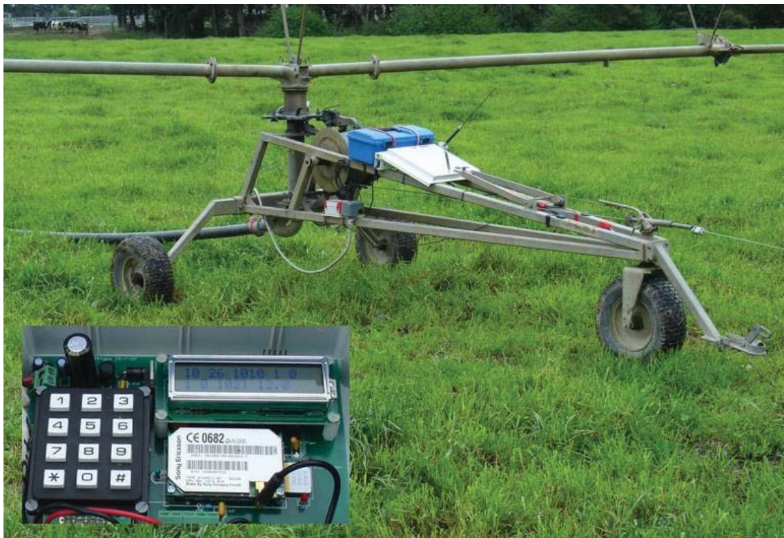
Plate 3.3 The small travelling irrigator (rotating boom) with the alert and remote sensing equipment installed at Massey University’s No.4 Dairy Farm (insert shows the combined cellular phone and GPS device).
