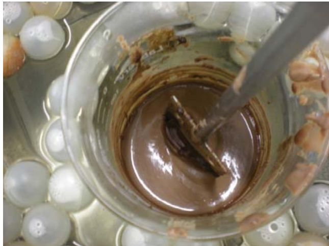
Figure 3.6: Qualitative observations during hydrolysis of beef: Hydrolysis conditions; 60°C, 2% w/w enzyme concentration.
