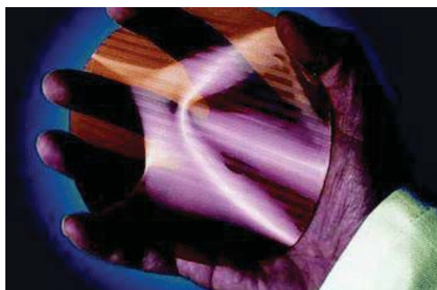
Figure 1.8 ORMOCER waveguides where the hybrid coating is deposited on a flexible foil. 51
