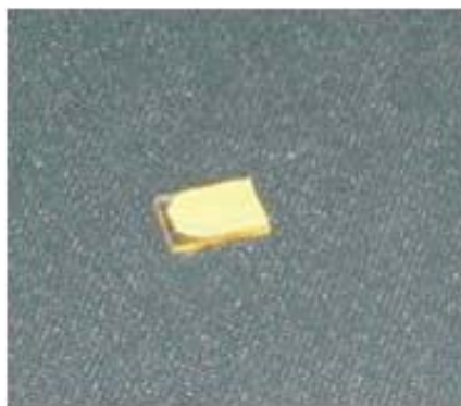
Figure 3.2 Polymer bound thick film of WO 3 -bpy coated on ITO glass substrate.
