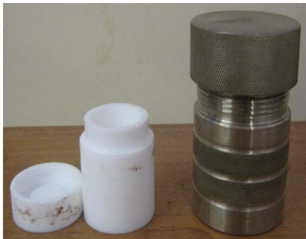
Figure 2.1 A stainless steel Teflon-lined autoclave used for synthesizing hybrid materials.
