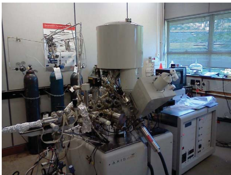
Figure 2.9 The Kratos Axis UltraDLD surface-analyzing chamber at the University of Auckland that was used for XPS measurements.
