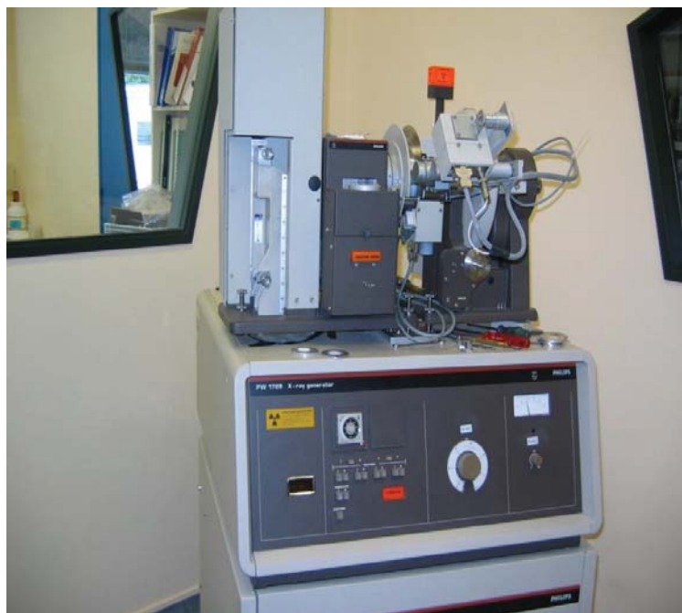
Figure 2.7 A powder X-ray diffractometer at Industrial Research, Lower Hutt was used for preliminary structural characterization of polycrystalline hybrid materials.
