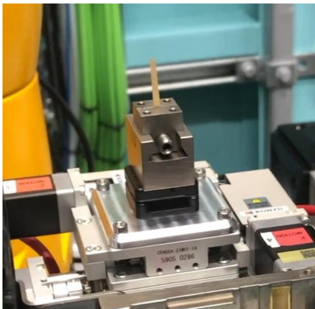
Figure 35 Composite sheet mounted on the sample platform in the MCT beamline (Australian Synchrotron).
